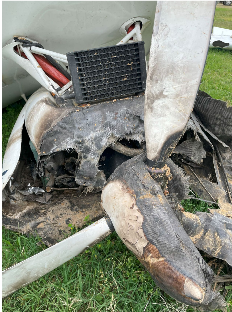
Photograph 4 - Closeup view of propeller damage. (NTSB)
