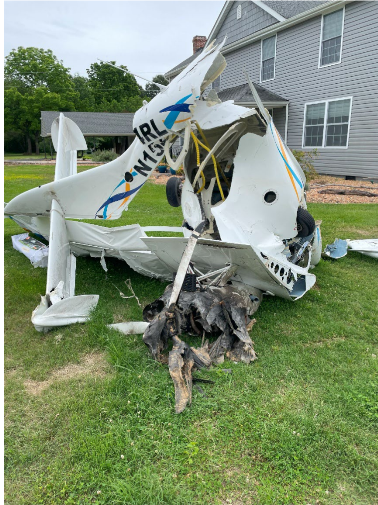
Photograph 1 - Overall view of airframe and engine wreckage. (NTSB)
