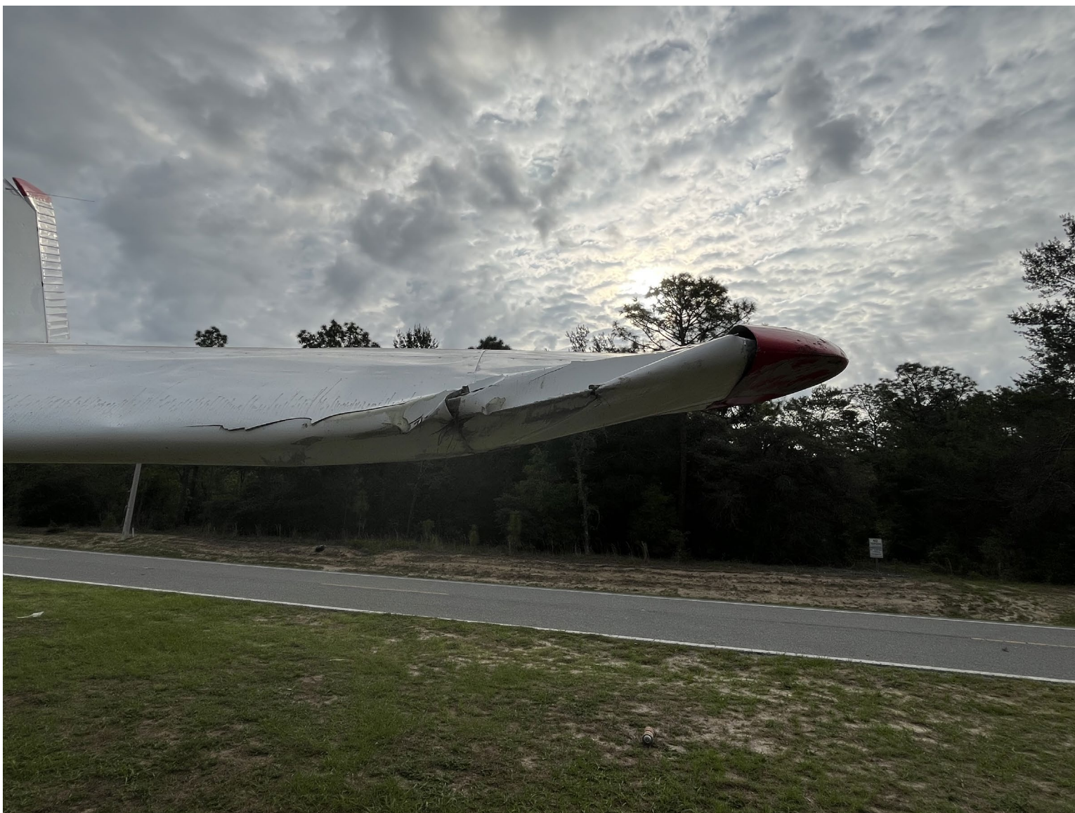
Photograph 2 - View of damage to the left wing. (Courtesy of FAA)
