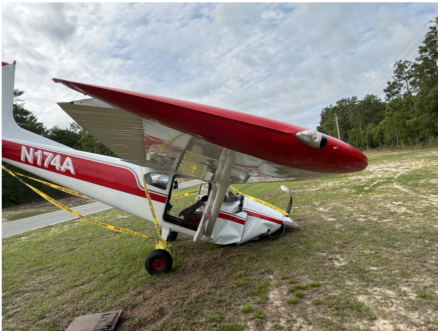
Photograph 3 - View of damage to the fuselage. (Courtesy of FAA)
