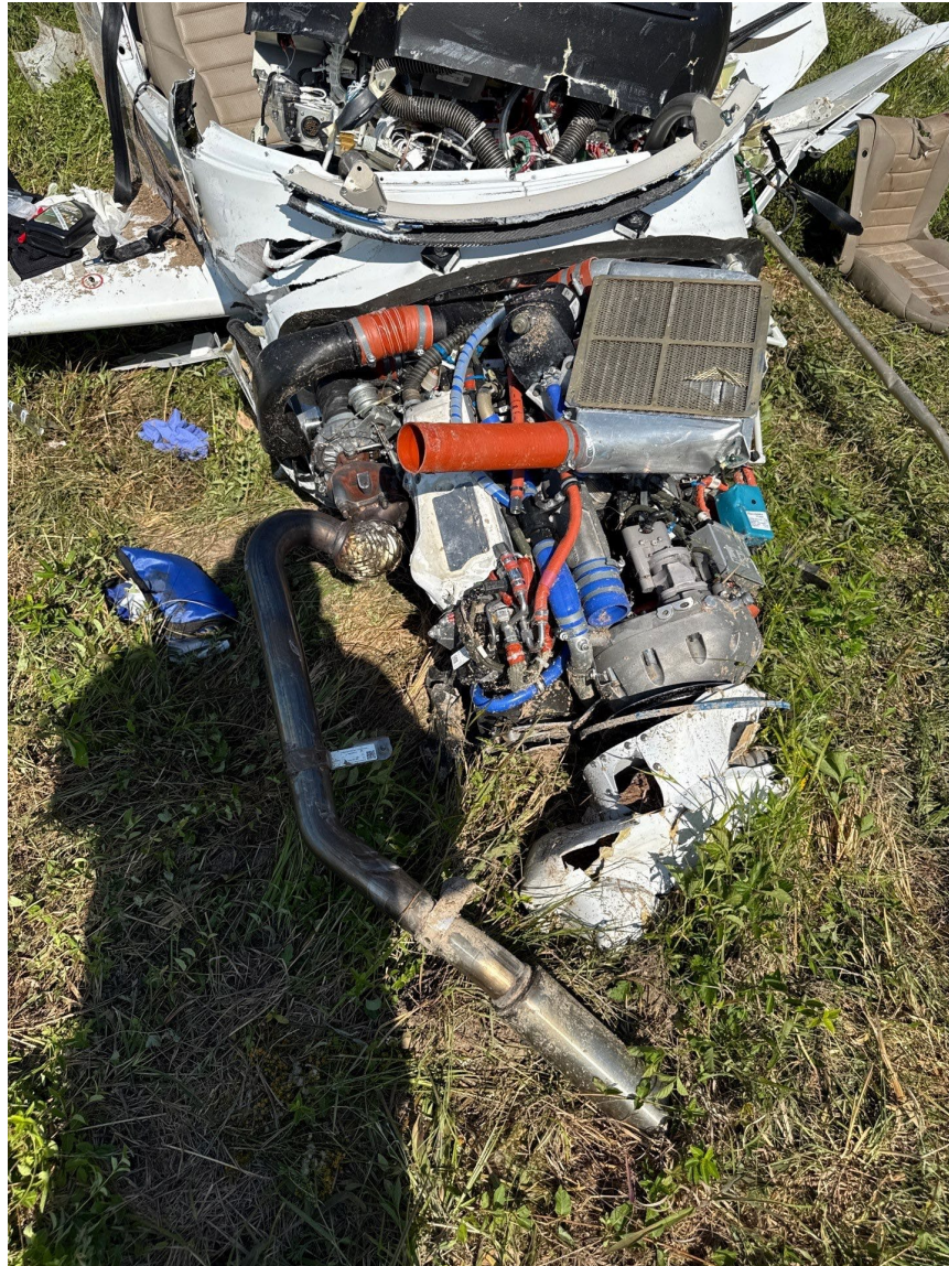
Photograph 3 - Engine, note: Air discharge duct missing. (Courtesy of FAA)
