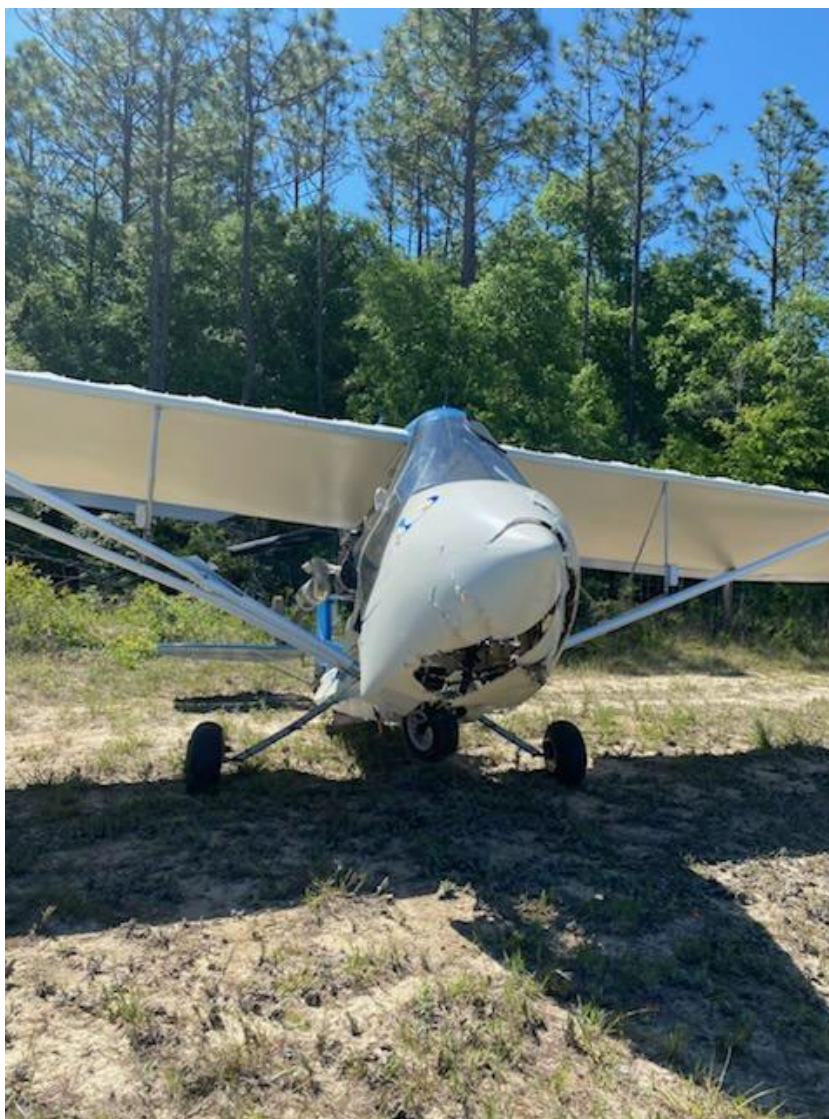
Photograph 2 - View of the Nose Hull Damage (Courtesy of FAA)
