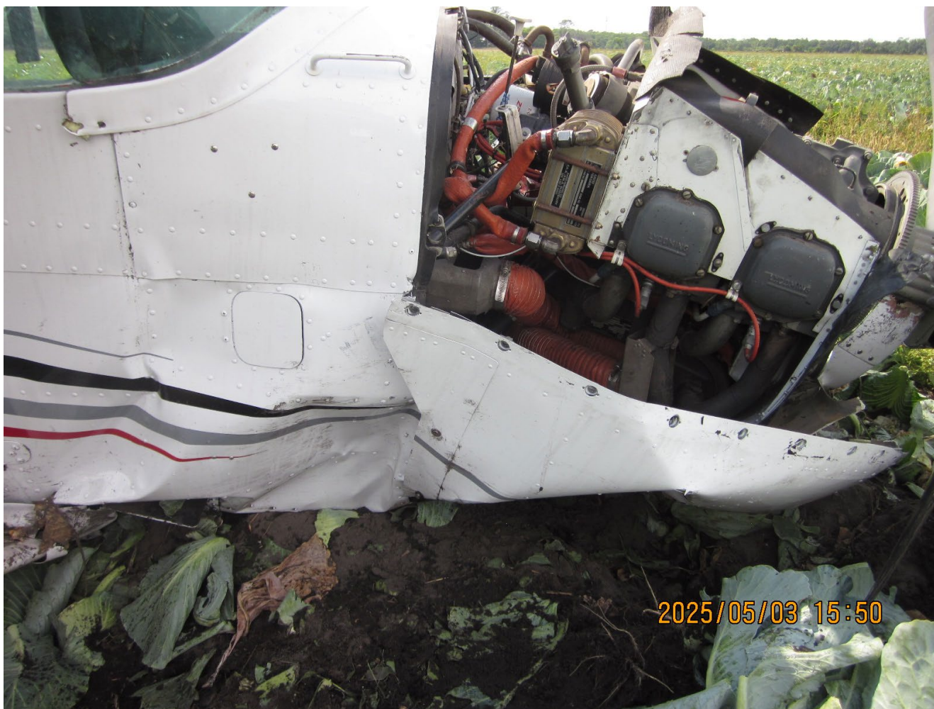
Photograph 3 - View of airframe and engine compartment damage. (Courtesy of FAA)
