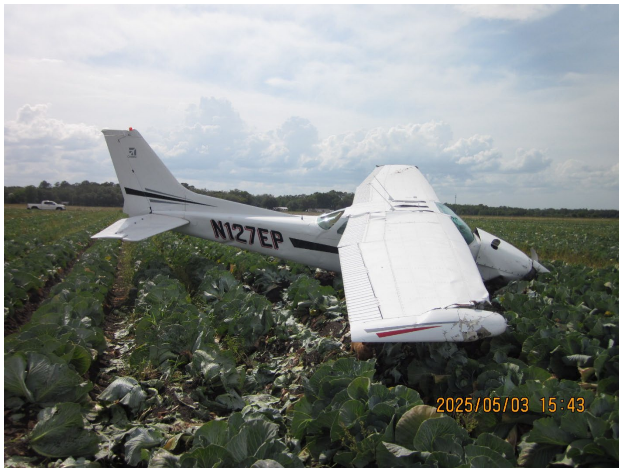
Photograph 1 - Right profile view of airplane at accident site. Note damage to right wing and engine compartment. (Courtesy of FAA)
