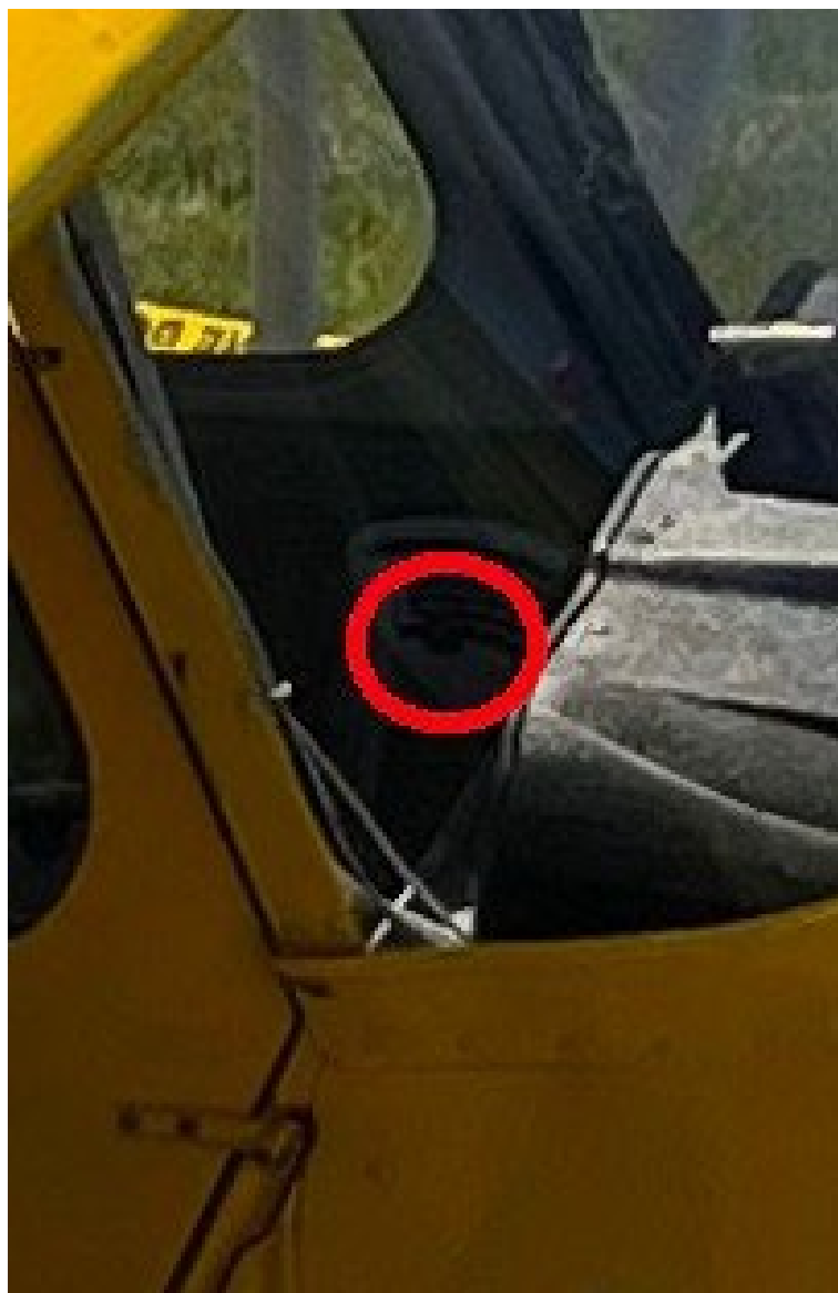
Photograph 2 - Main Wreckage Close-up [Carburetor Heat Control] (Courtesy of FAA)
