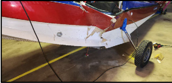
Figure 1 Left Side View Hull Damage
