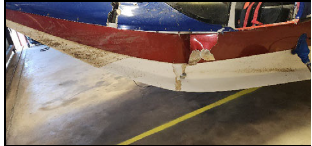
Figure 2 Right Side View Hull Damage
