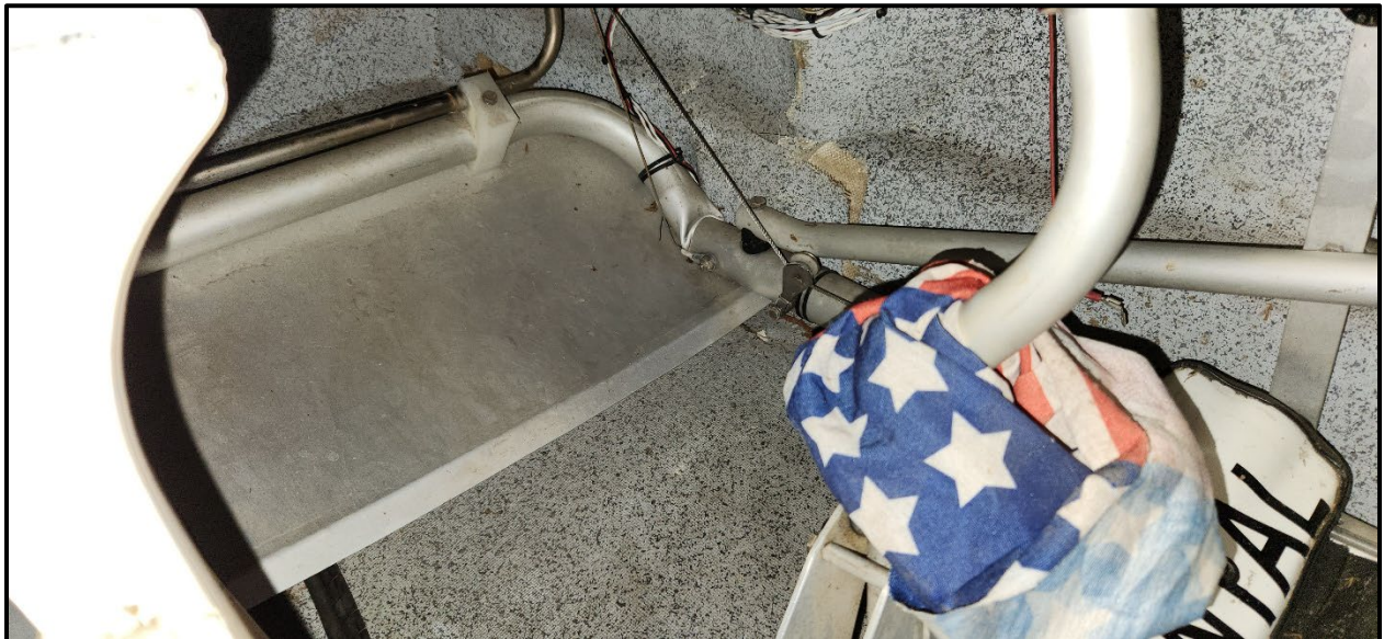
Figure 3 View of Cockpit Tube Damage
