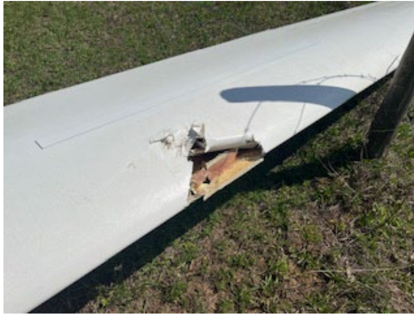
Photograph 4 - Damage to left wing (Source: Pilot)
