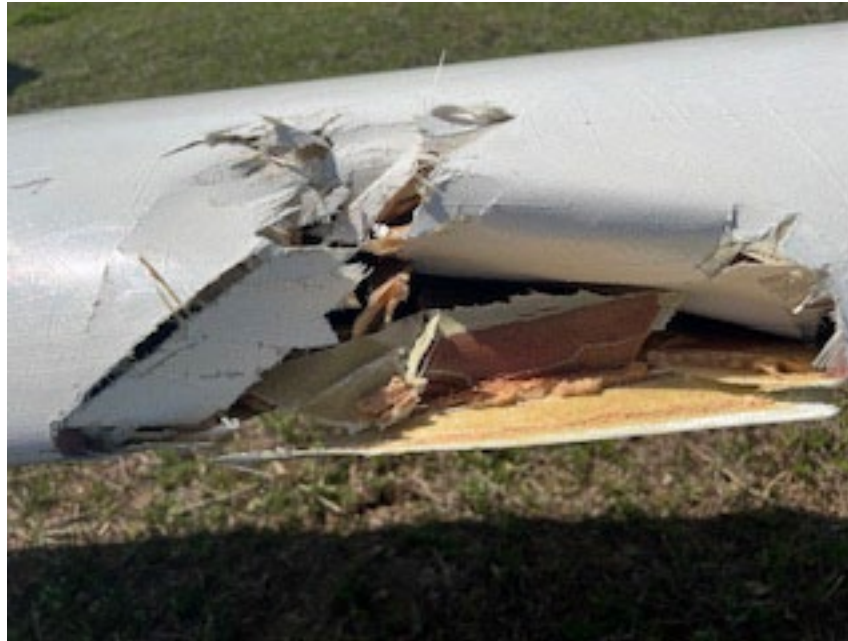
Photograph 5 - Damage to left wing (Source: Pilot)
