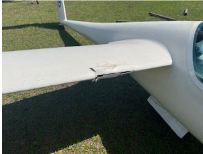
Photograph 3 - Damage to right wing (Source: Pilot)
