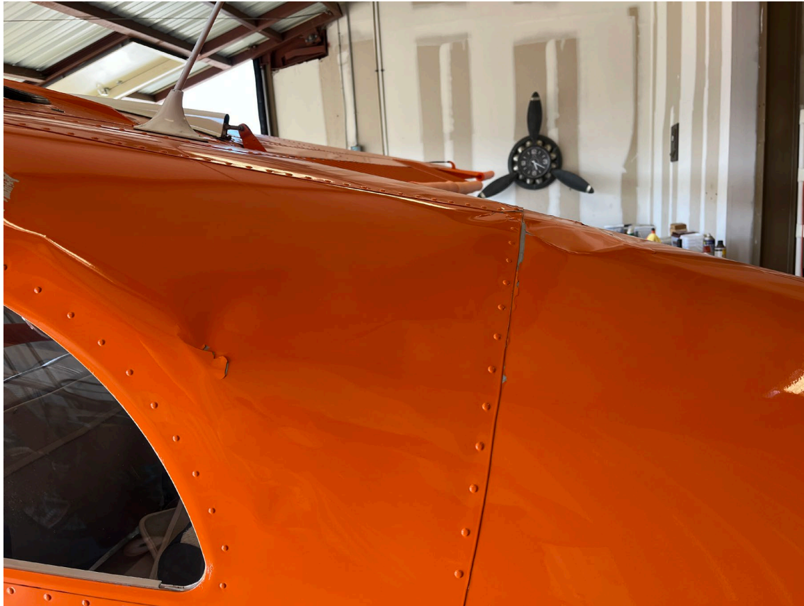
Photograph 1 - Upper fuselage accident damage (Courtesy of Pilot)
