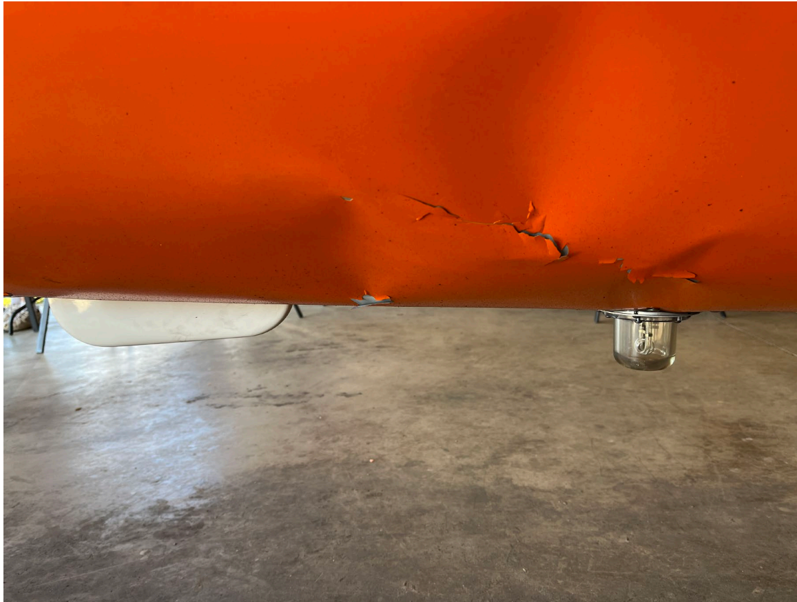
Photograph 2 - Lower fuselage accident damage (Courtesy of Pilot)
