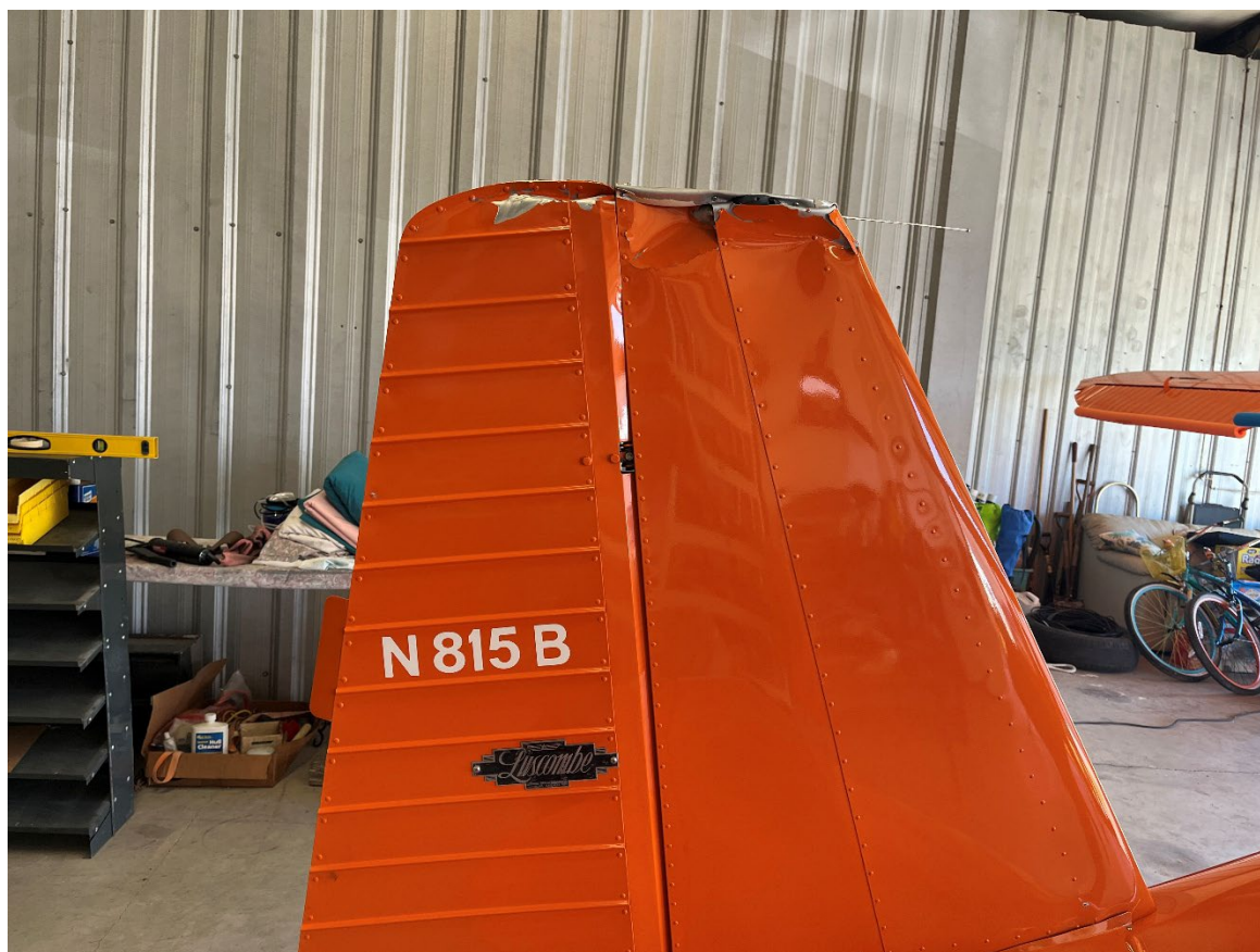
Photograph 3 - Vertical stabilizer and rudder accident damage (Courtesy of Pilot)
