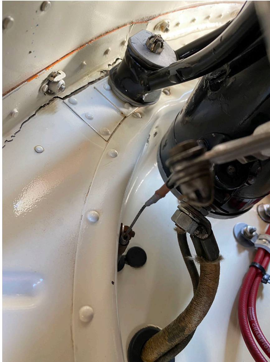
Photograph 4 - Engine mount and firewall structure accident damage (Courtesy of Pilot)
