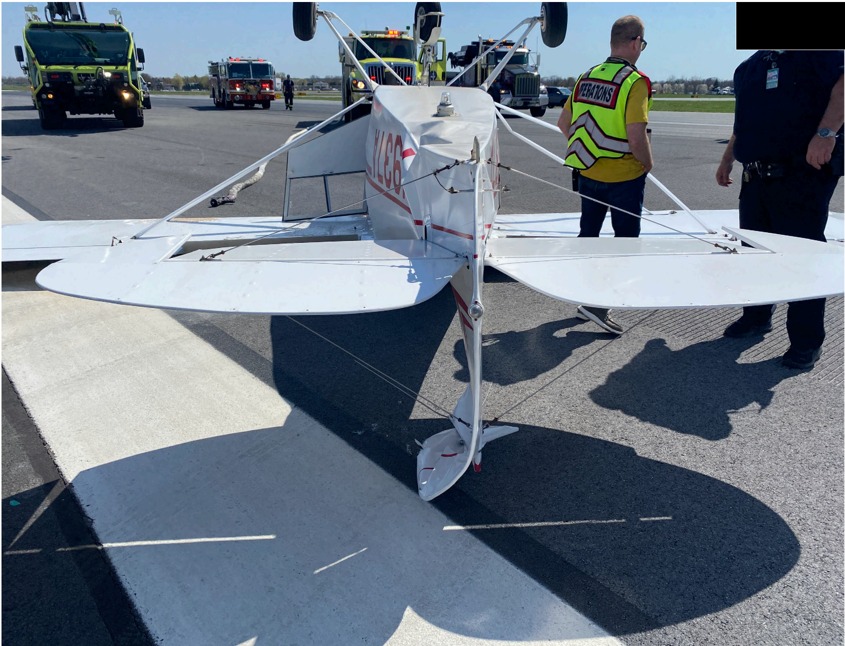
Photo 2 – View of Damage to Empennage and Vertical Fin as Found (FAA)
