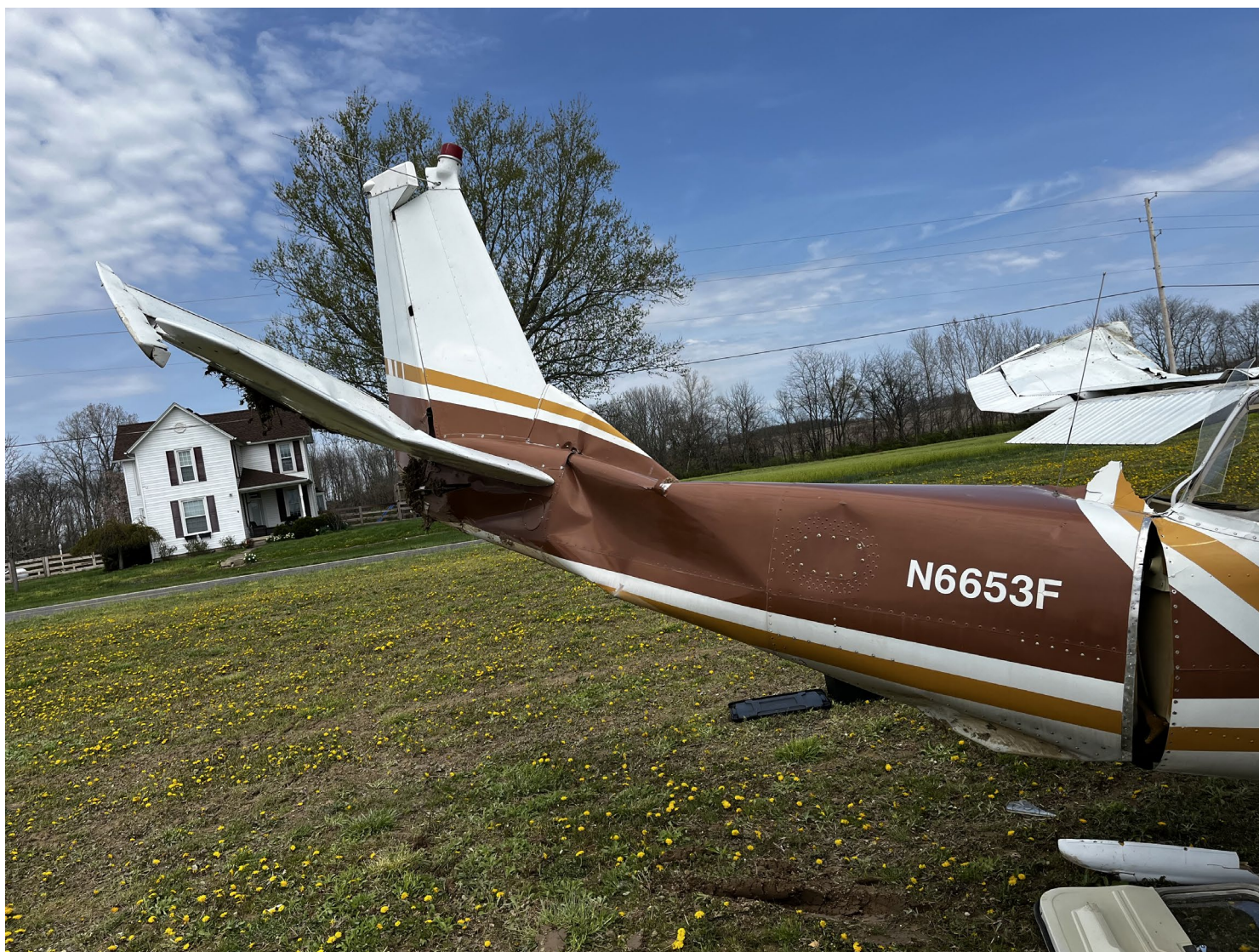
Photograph 2 - View of damage to the empennage. (Courtesy of FAA)
