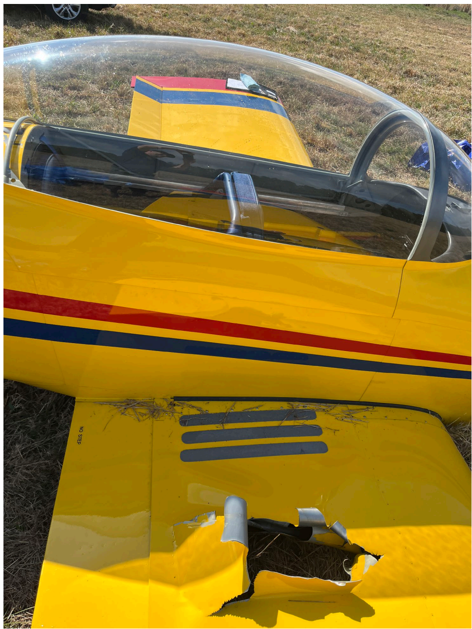
Photo 3 – View of Damage to Inboard Right Wing (FAA)
