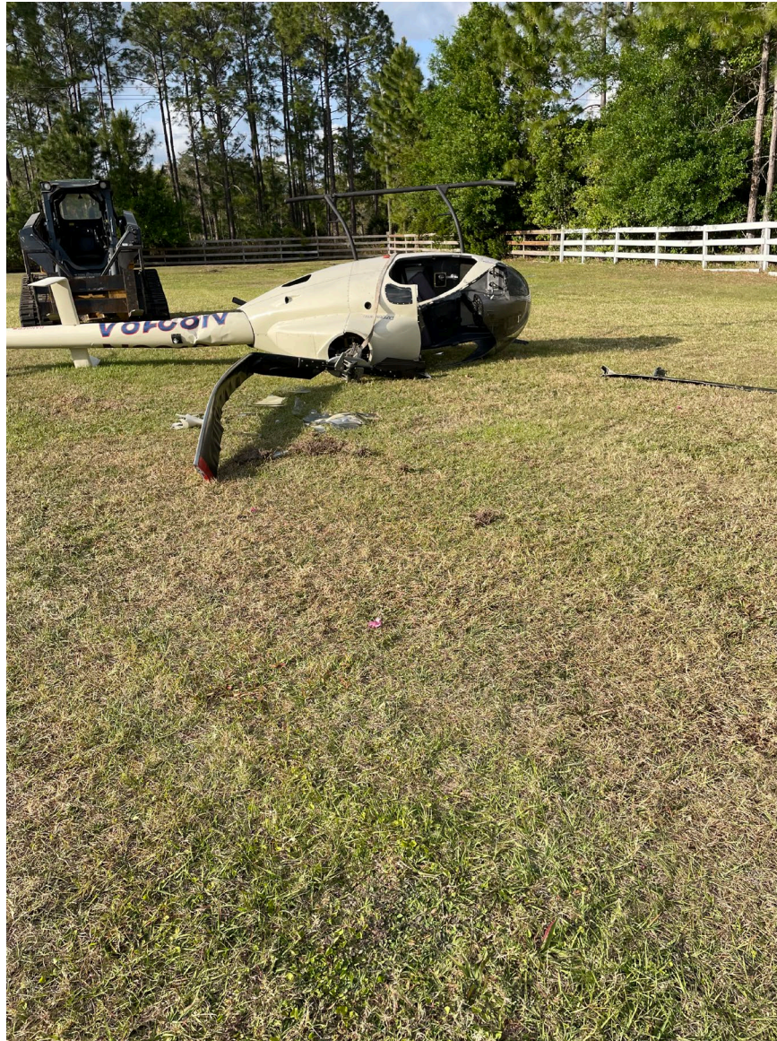
Photograph 1 - Deformation noted to main rotor blades (Courtesy of FAA)
