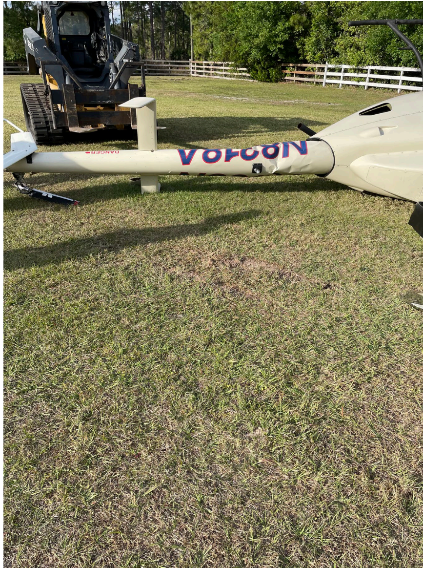
Photograph 2 - Deformation noted to tail boom (Courtesy of FAA)
