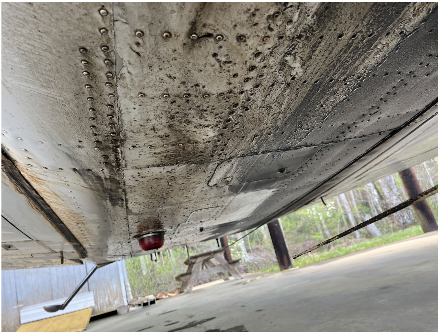
Photograph 4 - Bottom of fuselage covered in oil (Courtesy of FAA)
