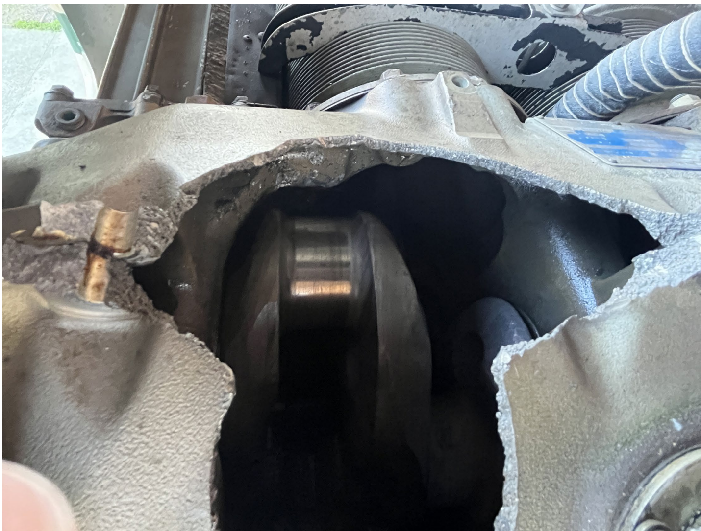
Photograph 2 - Hole in engine case (Courtesy of FAA)
