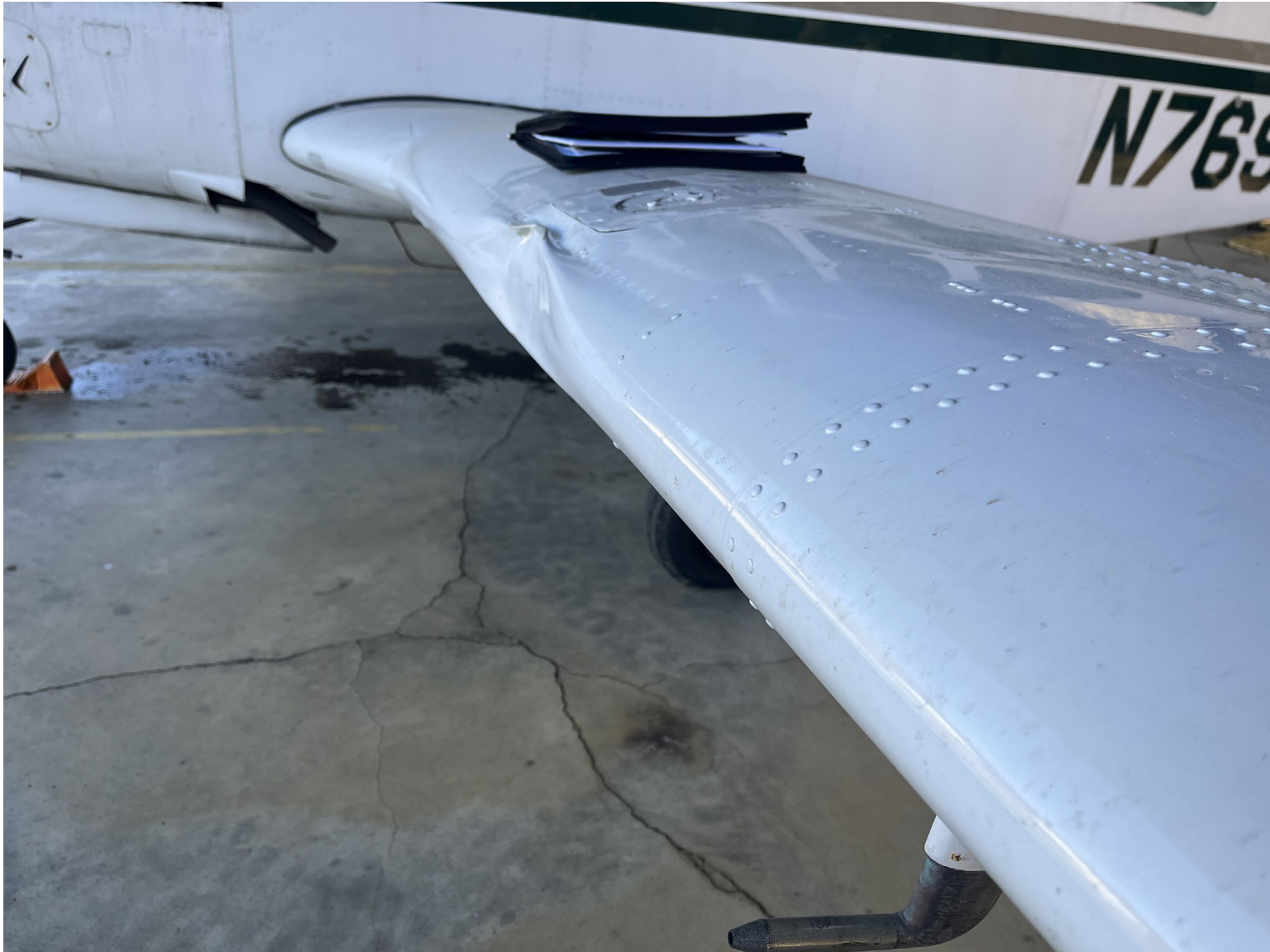
Photograph 1 - Left-Wing Leading-Edge Damage (Courtesy of FAA)
