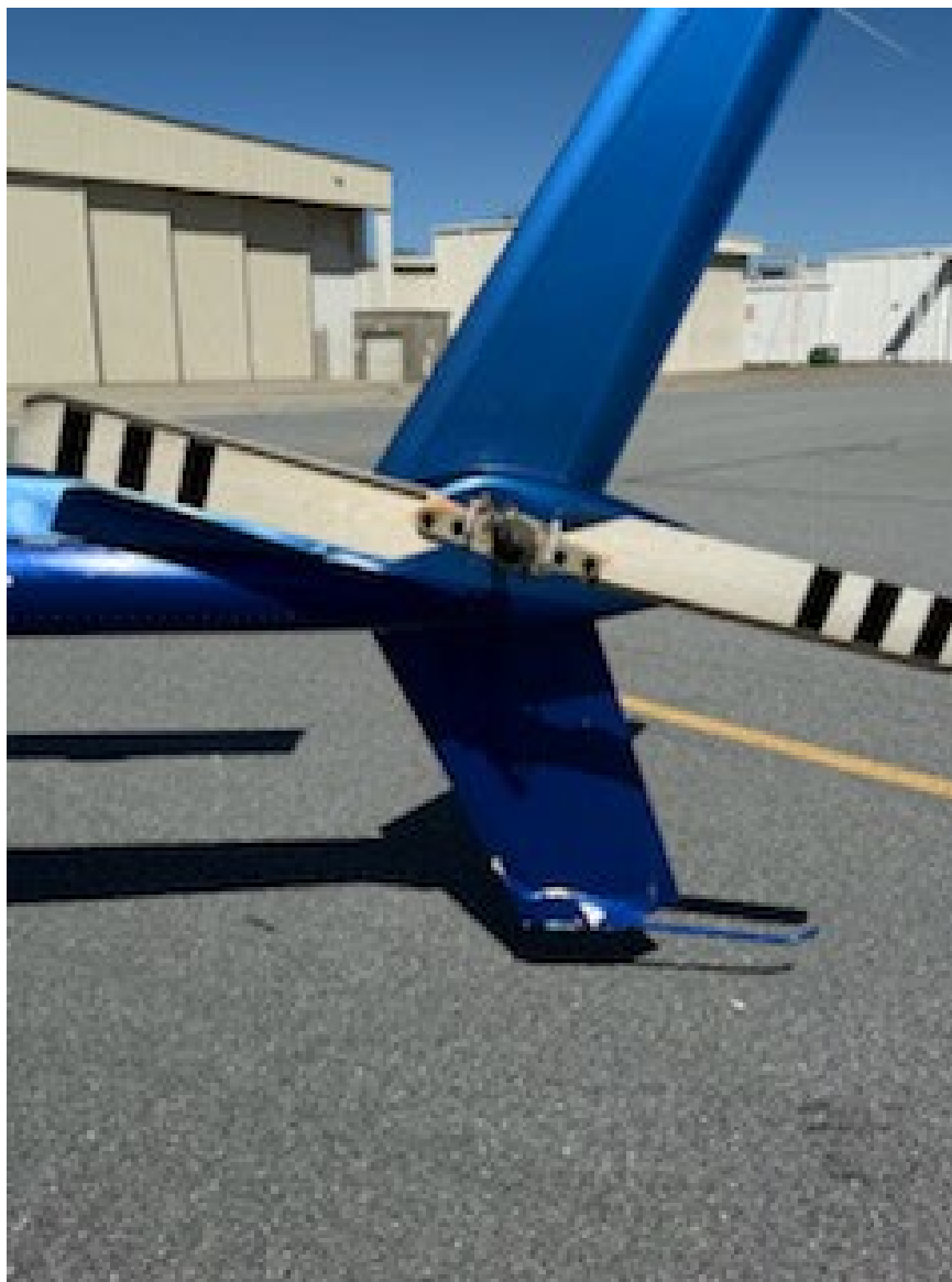
Photograph 5 - Vertical Fin Damage (Courtesy of FAA)
