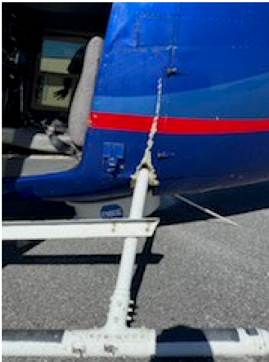
Photograph 2 - Left Side Fuselage Damage (Courtesy of FAA)
