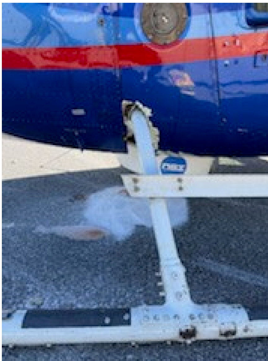
Photograph 4 - Closeup of Right Side Fuselage Damage (Courtesy of FAA)
