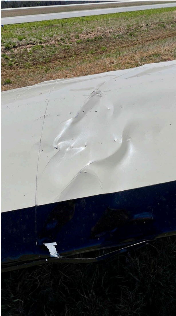
Photograph 2 - View of wing damage. (Courtesy of FAA)
