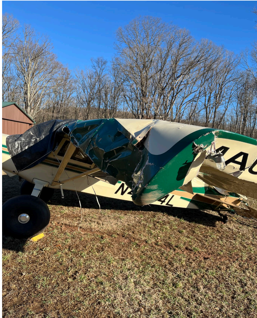
Photograph 2 - View of green and white airplane left side buckled wing. (Courtesy of FAA)
