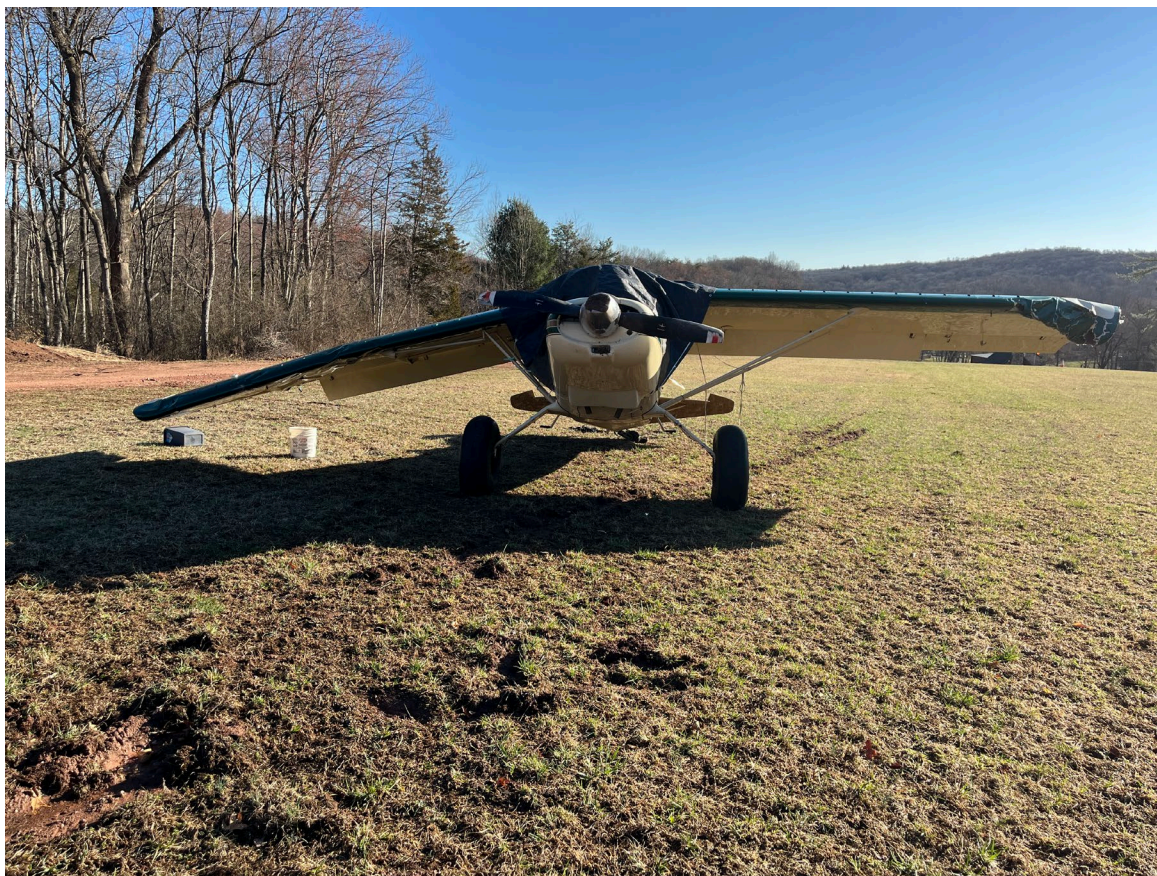
Photograph 1 - Front view of green and white airplane showing buckled wings (Courtesy of FAA)
