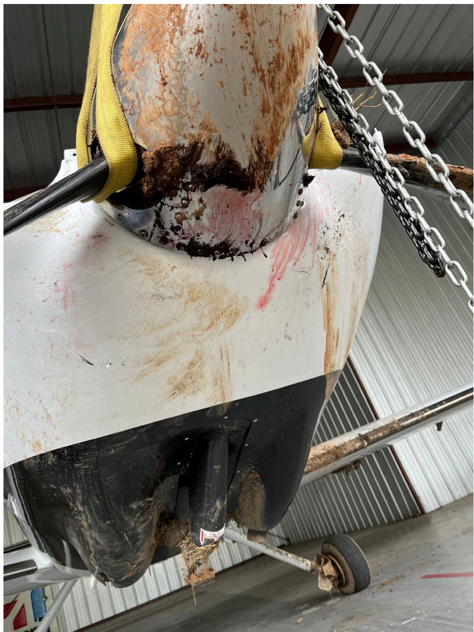
Photo 2 – View of Bent Nose Landing Gear Mount and Surrounding Structure (FAA)
