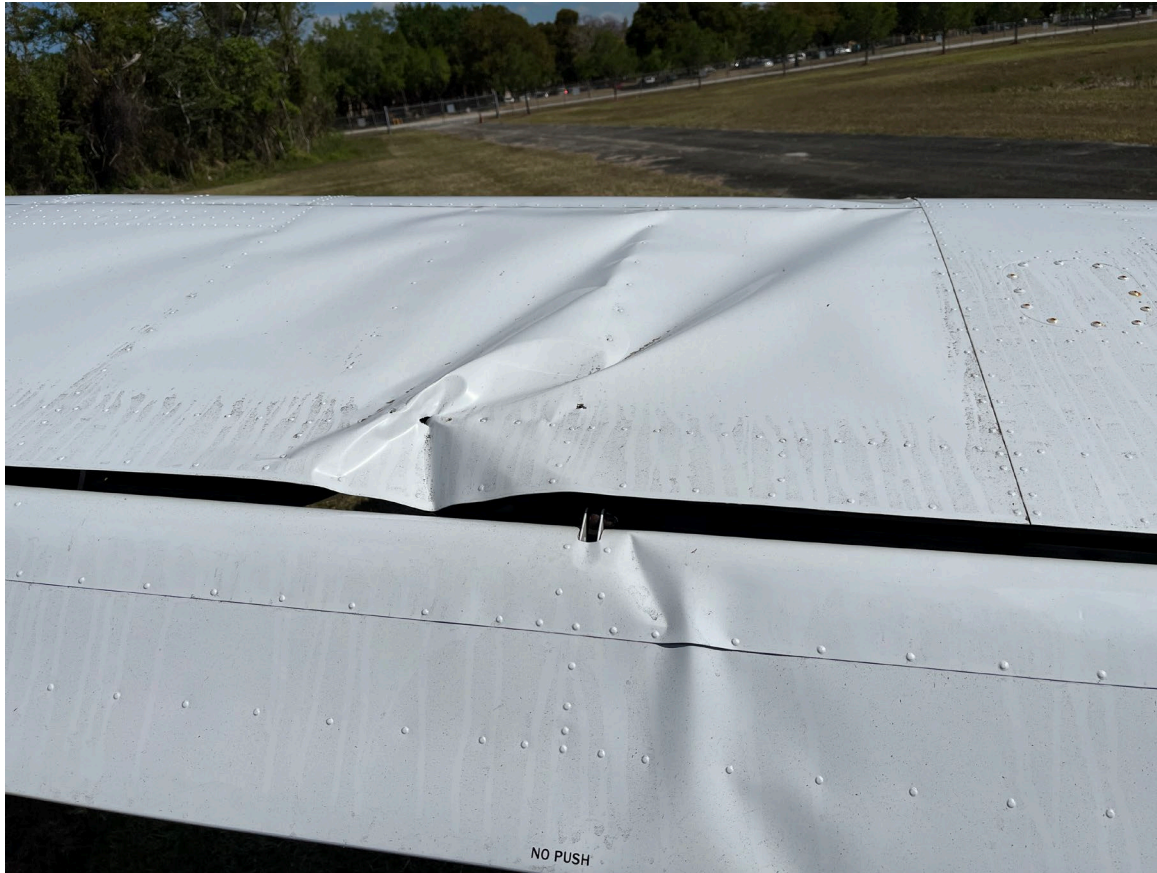
Photograph 2 - Deformation noted to left wing structure (Courtesy of FAA)
