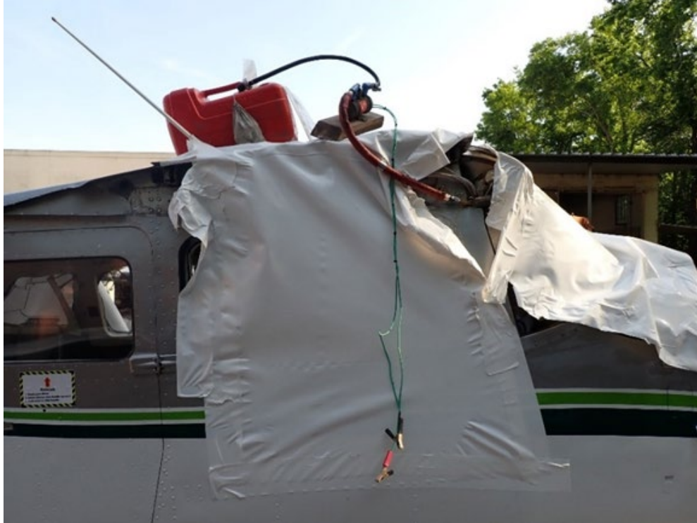
ASI-25-BB-081 – Small Fuel Container with Aviation Gasoline 100LL Plumbed to Right Wing Root
