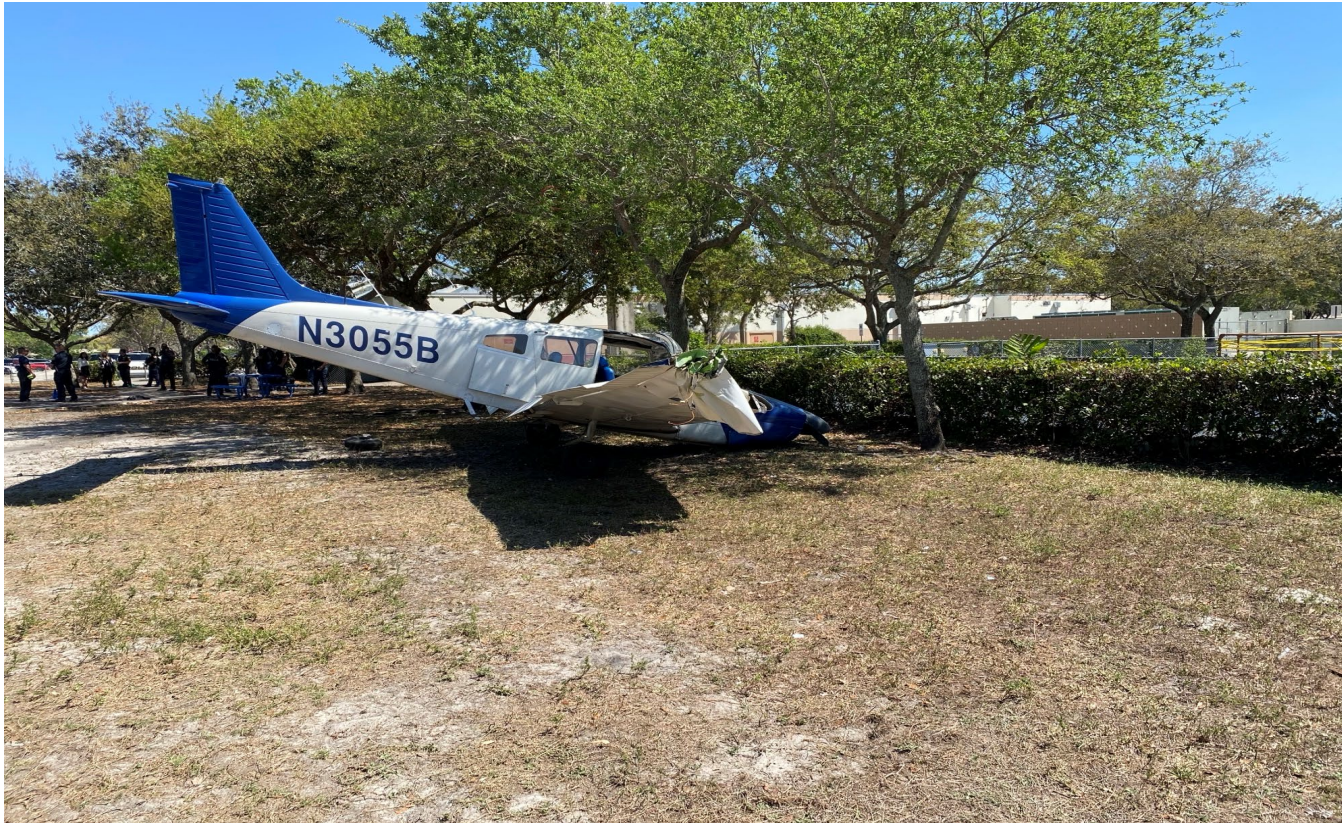
Photograph 1 - View of right side of airplane showing damaged right wing. (Courtesy of FAA)
