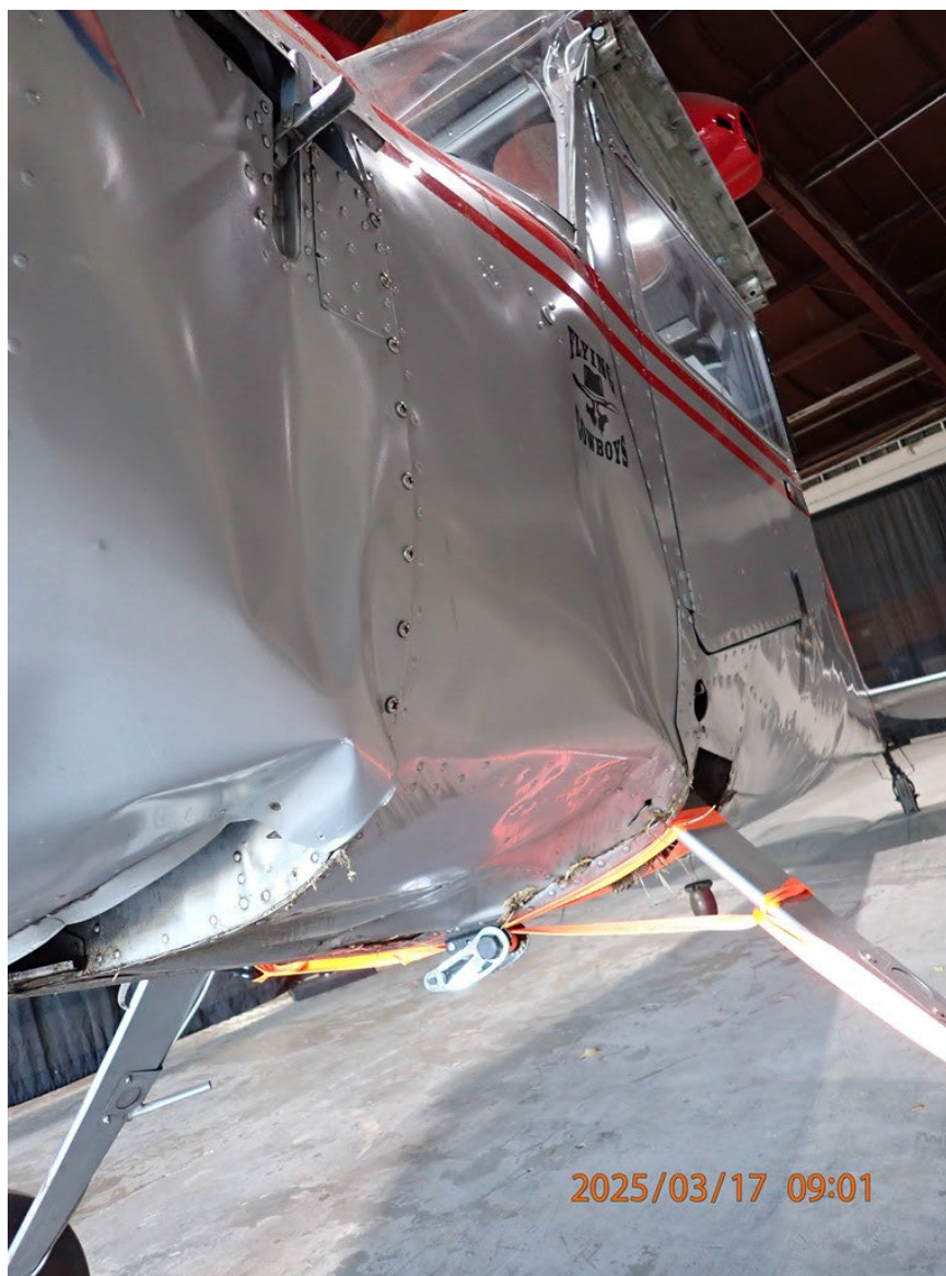
Photograph 3 -Fuselage Damage (Courtesy of NTSB)
