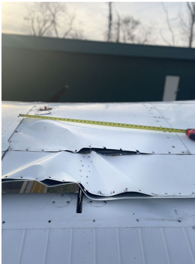
Photograph 10 - Close Up of Wing Fuselage Juncture (Courtesy of FAA)
