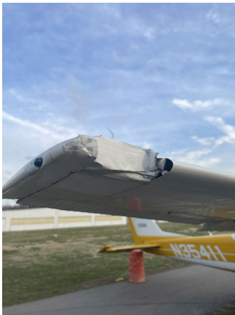
Photograph 12 - Right Wing Outboard Leading Edge (Courtesy of FAA)
