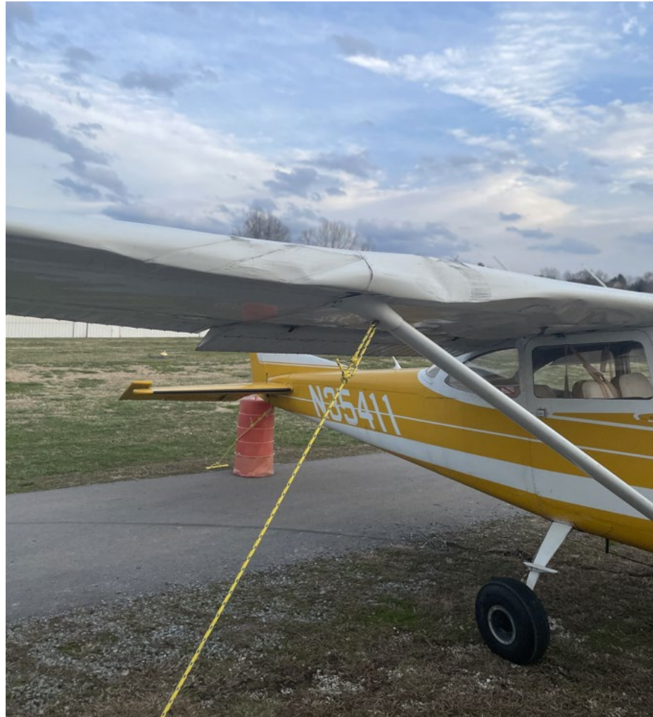
Photograph 13 - Right Wing Mid-Span Leading Edge (Courtesy of FAA)
