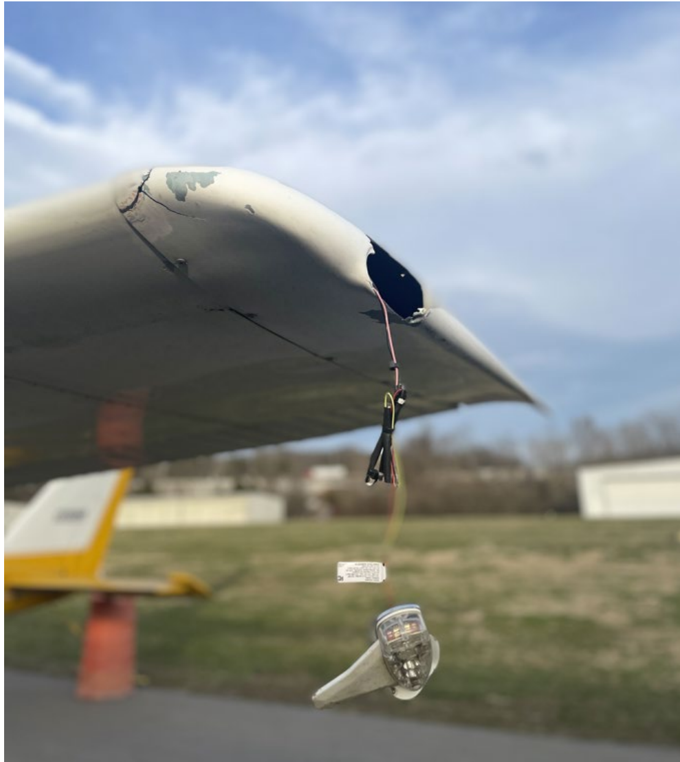
Photograph 8 - Left Wing Tip (Courtesy of FAA)
