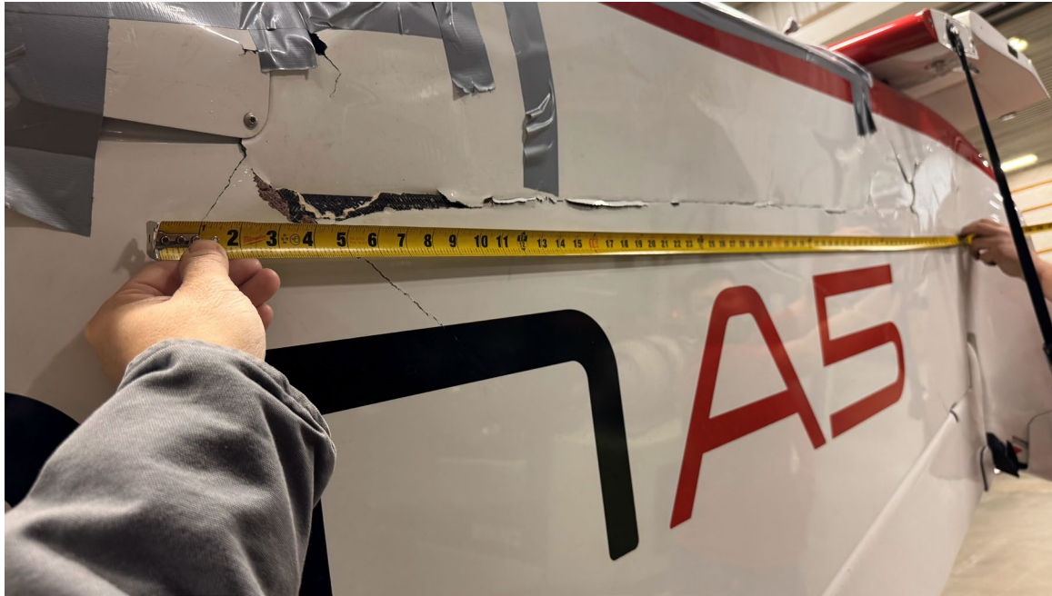
Photograph 2 - Right side fuselage accident damage (Courtesy of maintenance)
