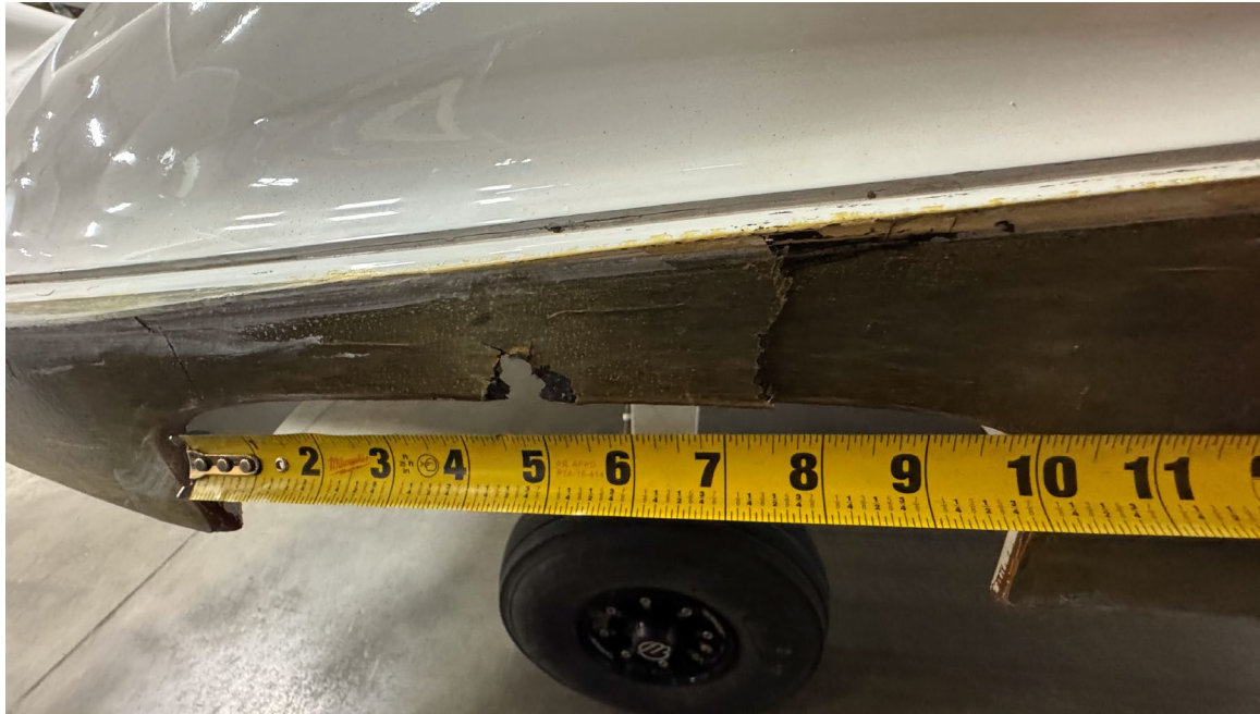
Photograph 3 - Right main landing gear pylon accident damage (Courtesy of maintenance)
