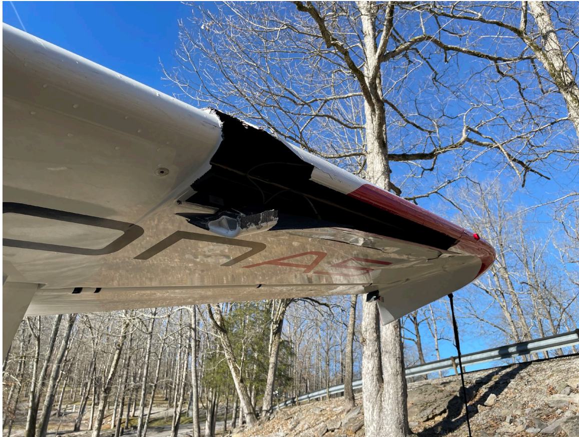
Photograph 4 - Left wing accident damage (Courtesy of FAA)
