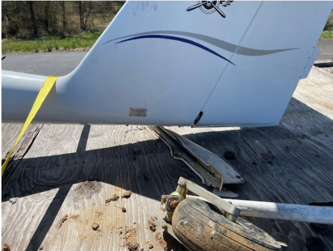
Photograph 3 - Lower vertical stabilizer accident damage (Courtesy of Flight School)
