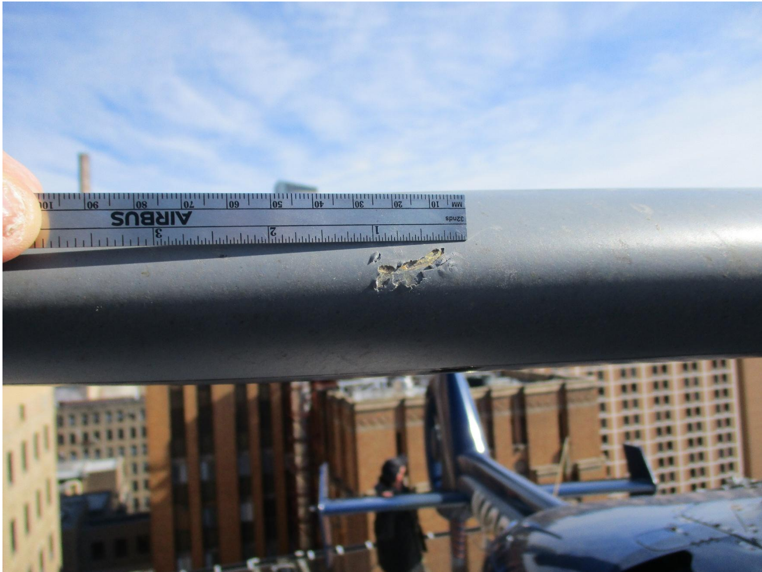
Photograph 1 - Damage to main rotor (Courtesy of FAA)
