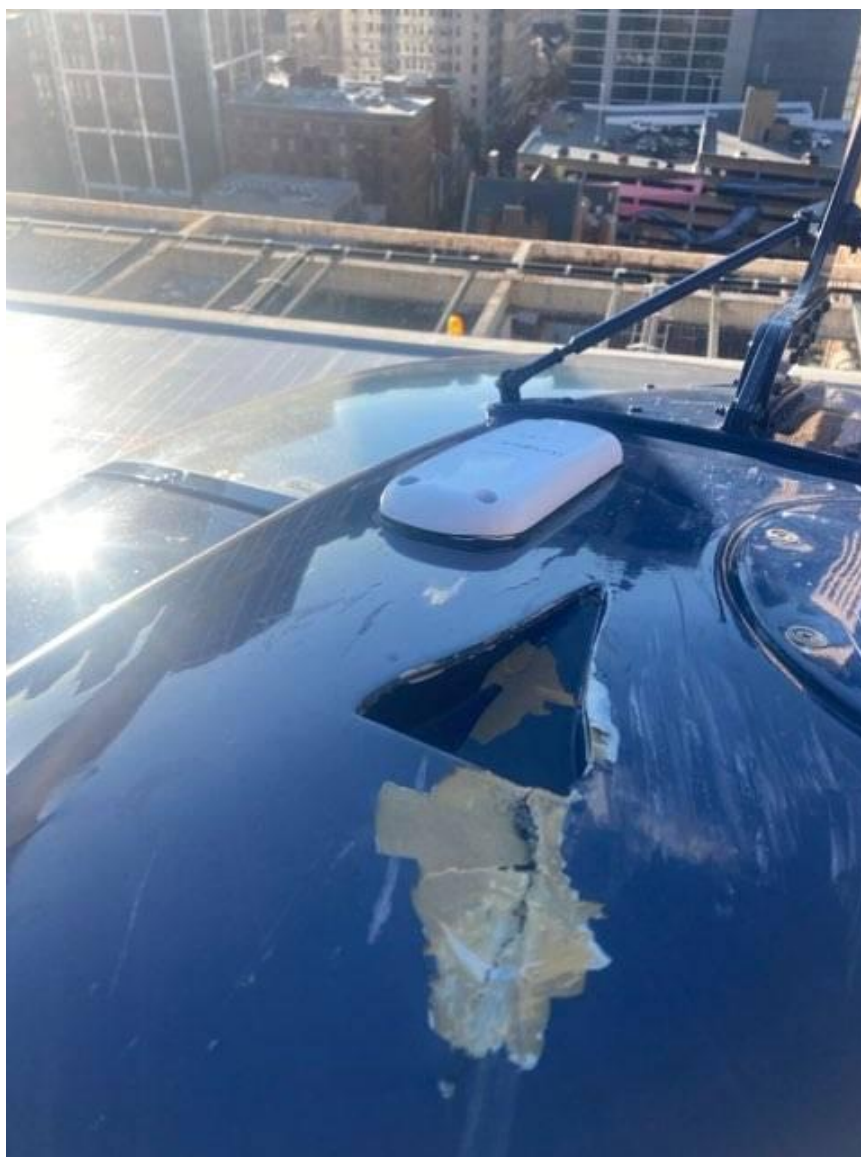
Photograph 2 - Damage to helicopter (Courtesy of FAA)
