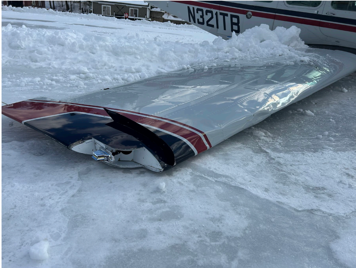
Photograph 3 – View of right wing of airplane showing buckling damage (Courtesy of FAA)
