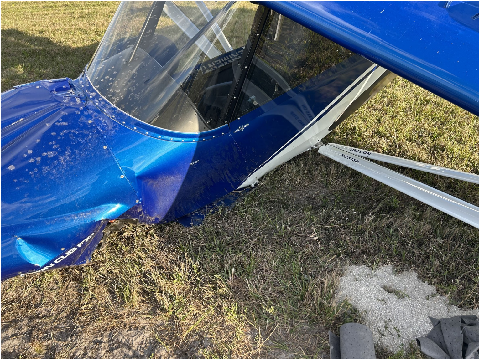
Photograph 1 - Left gear collapsed, folded under fuselage (Courtesy of Owner)
