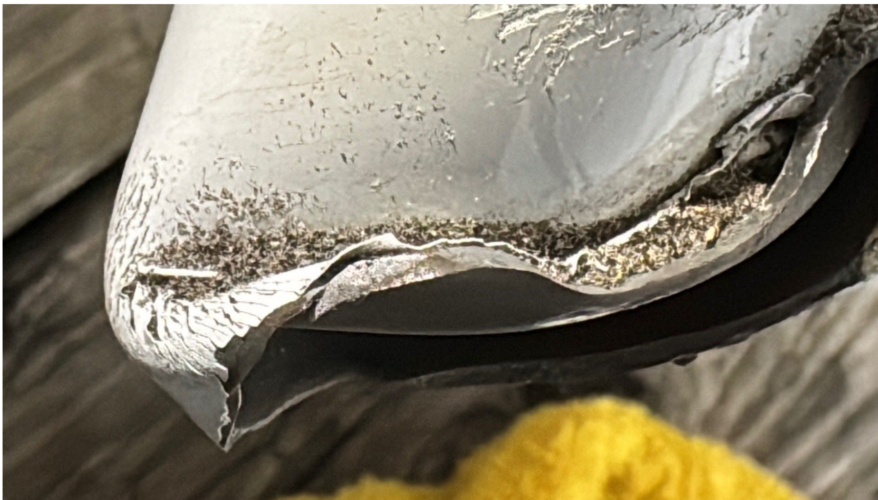
Photograph 6 - Left landing gear tube (Courtesy of FAA)
