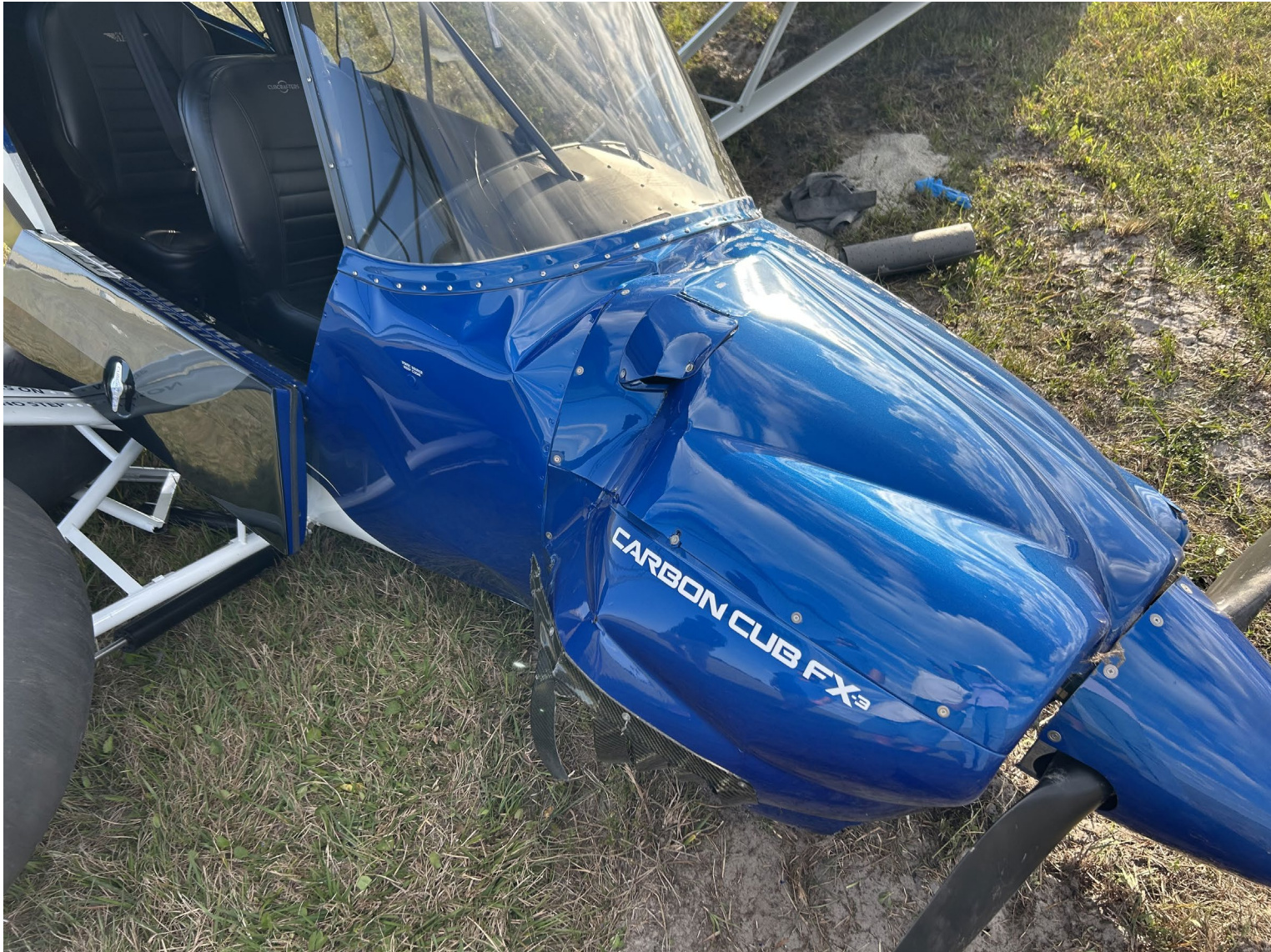
Photograph 3 - Front of aircraft and firewall damage (Courtesy of Owner)
