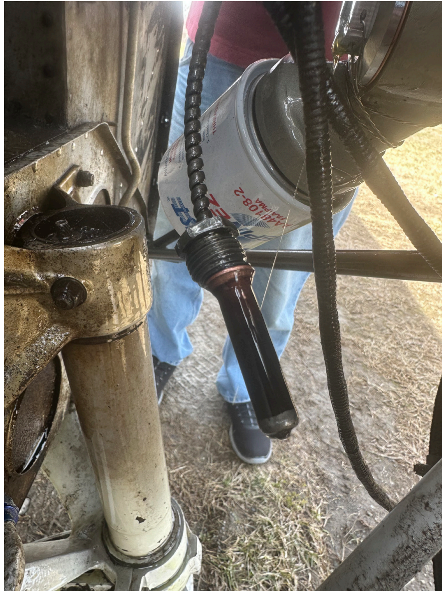
Photograph 3 - Oil temperature probe (Courtesy of Owner/Pilot)
