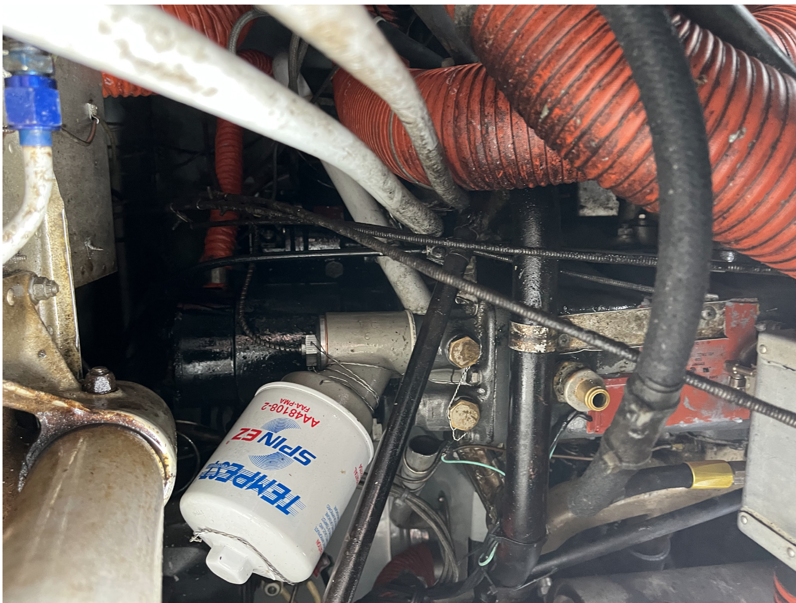
Photograph 2 - Oil filter and adapter (Courtesy of FAA)
