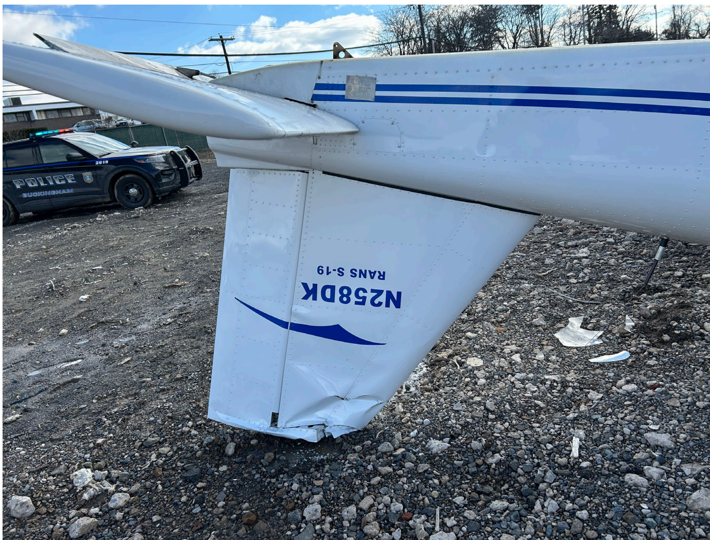
Photograph 2 - Vertical stabilizer accident damage (Courtesy of FAA)
