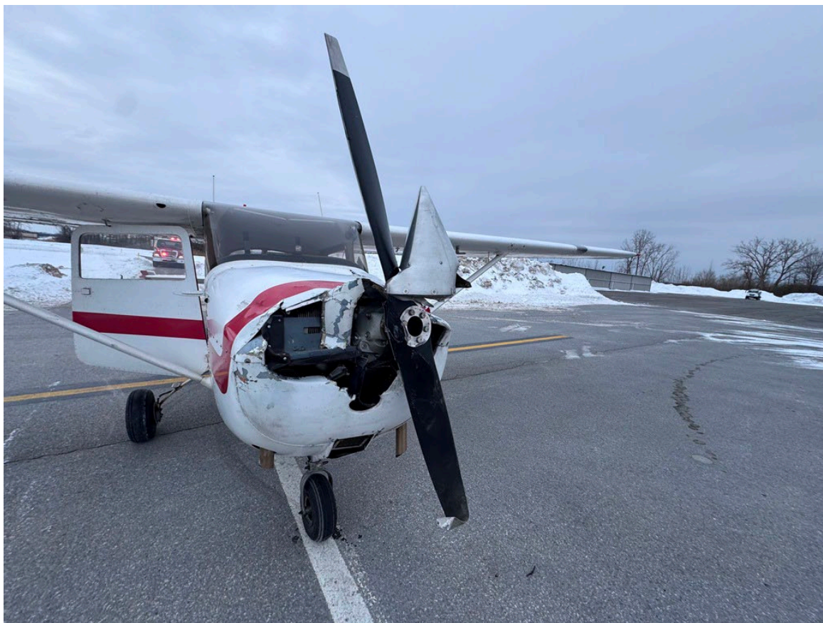
Photograph 1 - Front View of Airplane Damage (Courtesy of C. Blas)
