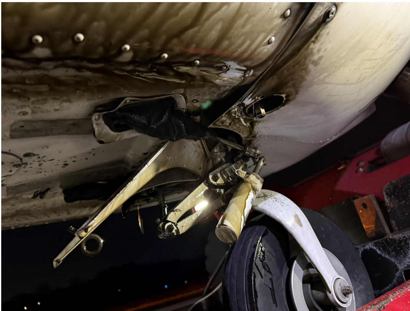
Photograph 4 - Damage Behind Firewall (Courtesy of FAA)
