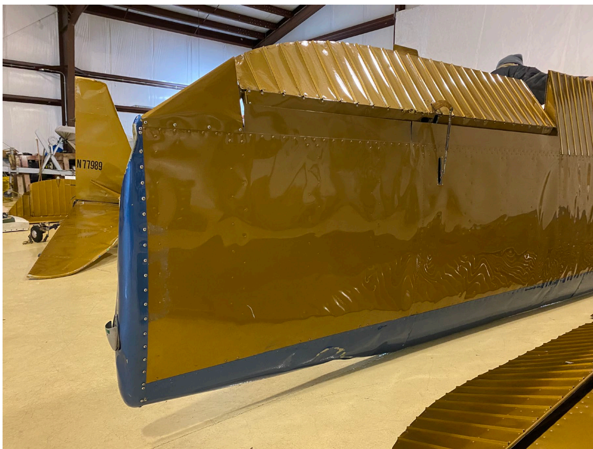
Photograph 2 - Right Wing Accident Damage (Courtesy of Pilot)
