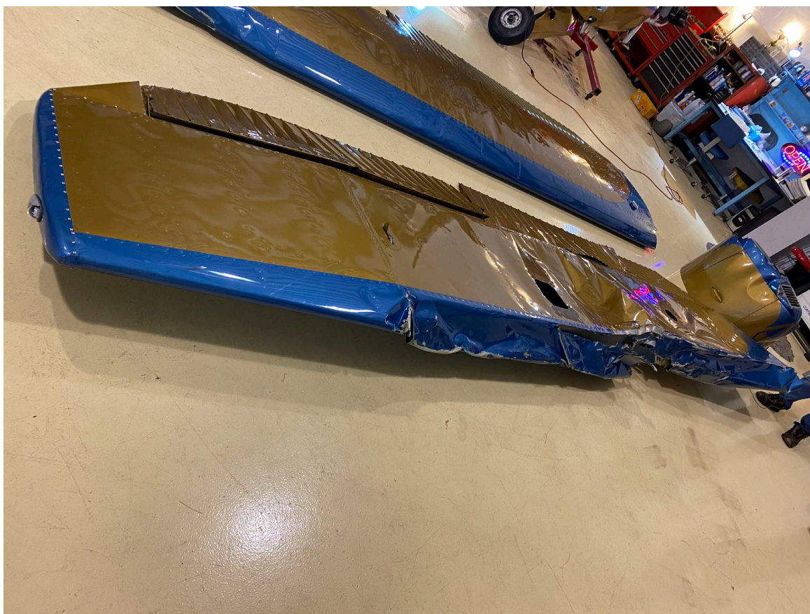
Photograph 1 - Left Wing Accident Damage (Courtesy of Pilot)
