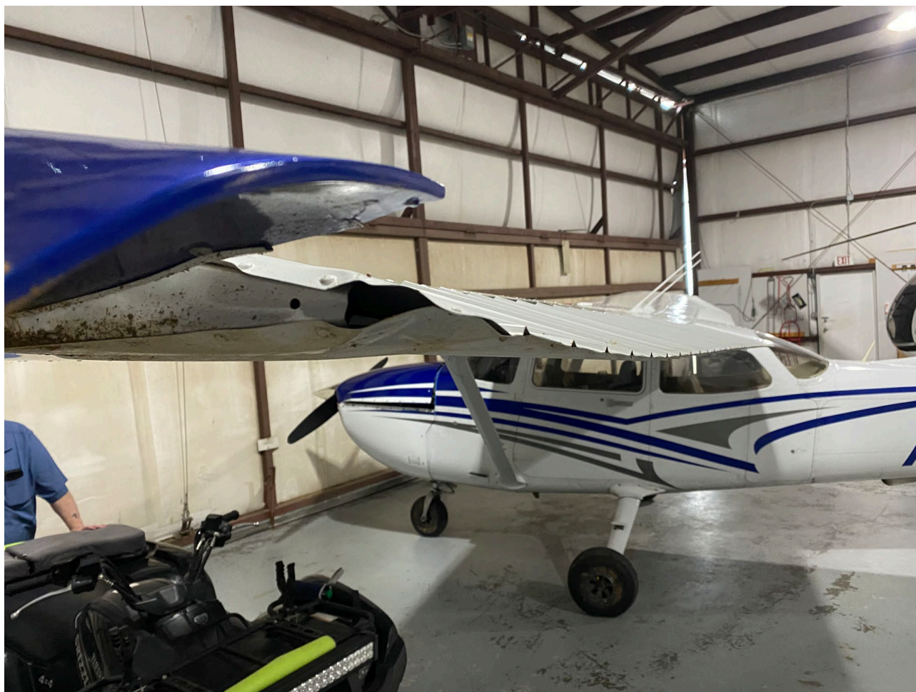
Photograph 1 - View of damaged left wing. (Courtesy of FAA)
