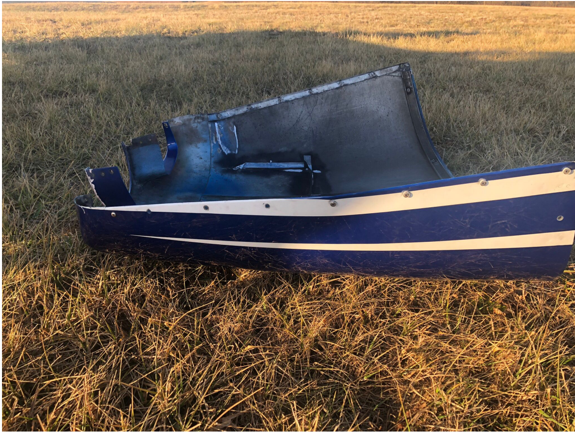
Picture 2: Cowling condition after landing, some screws missing possibly during detachment.
