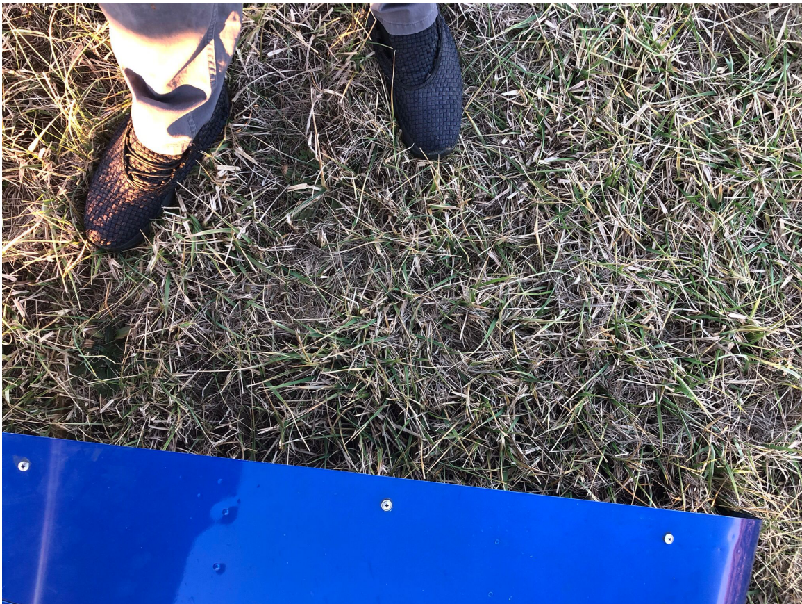
Picture 3: Cowling condition after landing – all 3 screws on top of cowling present.
