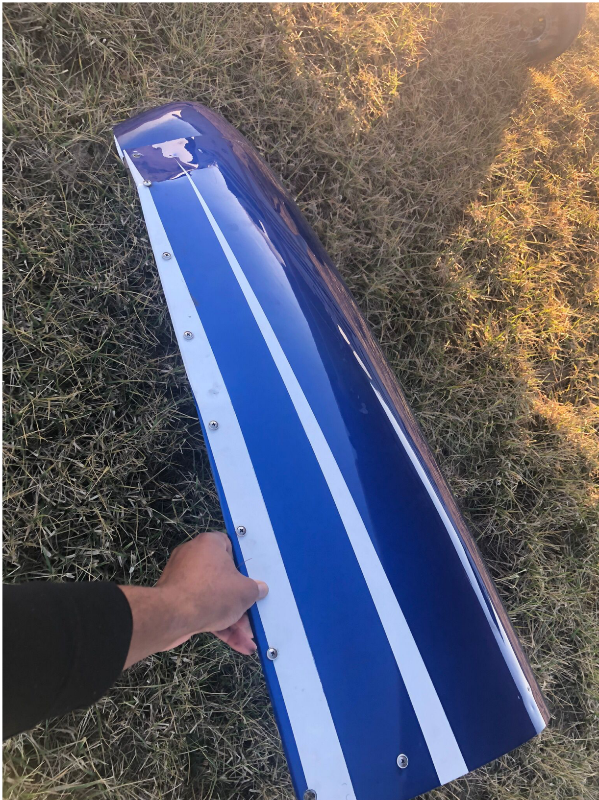
Picture 1: Cowling condition after landing – most screws still in place.
