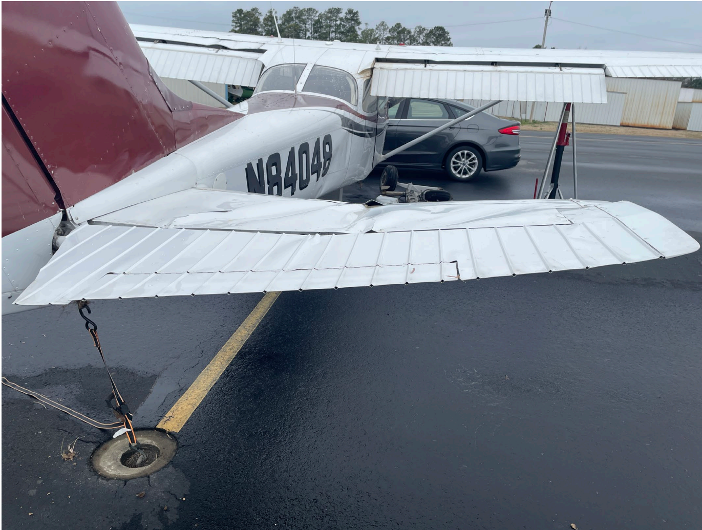
Photograph 3 - Right horizontal stabilizer and elevator accident damage (Courtesy of FAA)
