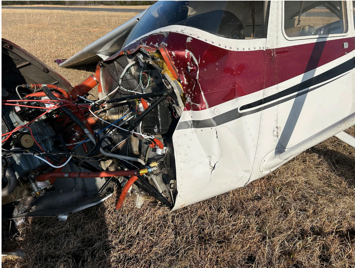
Photograph 5 - Forward fuselage accident damage (Courtesy of FAA)
