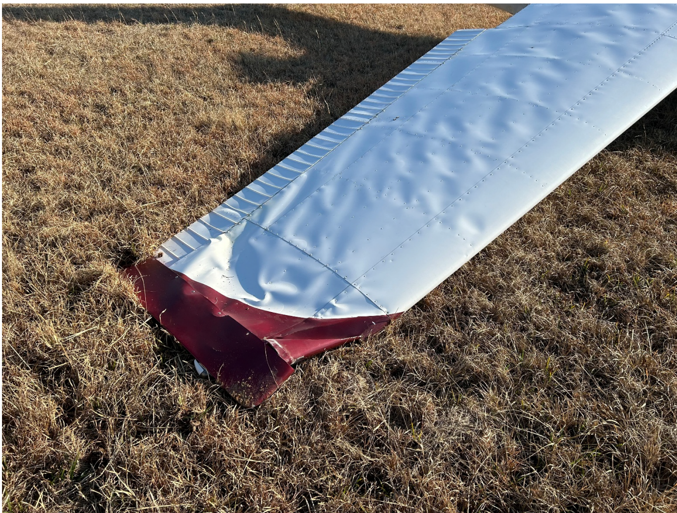
Photograph 2 - Right wing accident damage (Courtesy of FAA)
