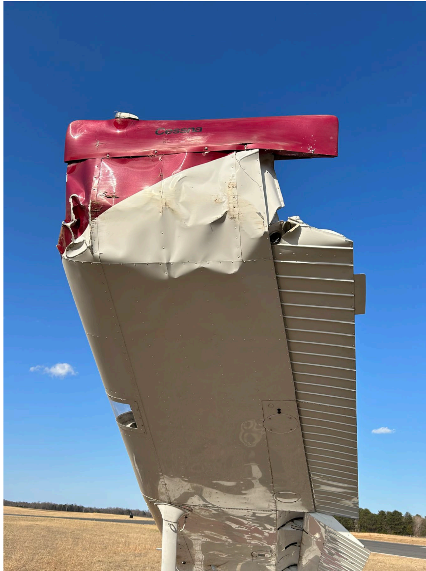
Photograph 4 - Left wing accident damage (Courtesy of FAA)
