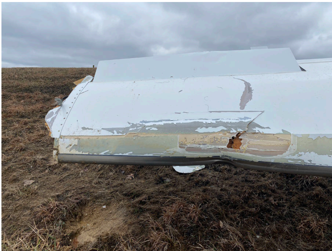
Photograph 6 - FAA Digital Photograph. Frontal View of the Outer Section of the Right Wing Showing Substantial Damage
