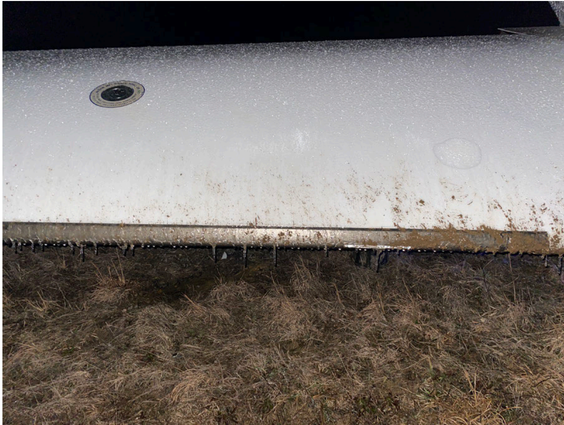
Photograph 5 - FAA Digital Photograph. View of a portion of the Right Wing. Note Dirt on the Leading Edge on Top of a Layer of Ice
