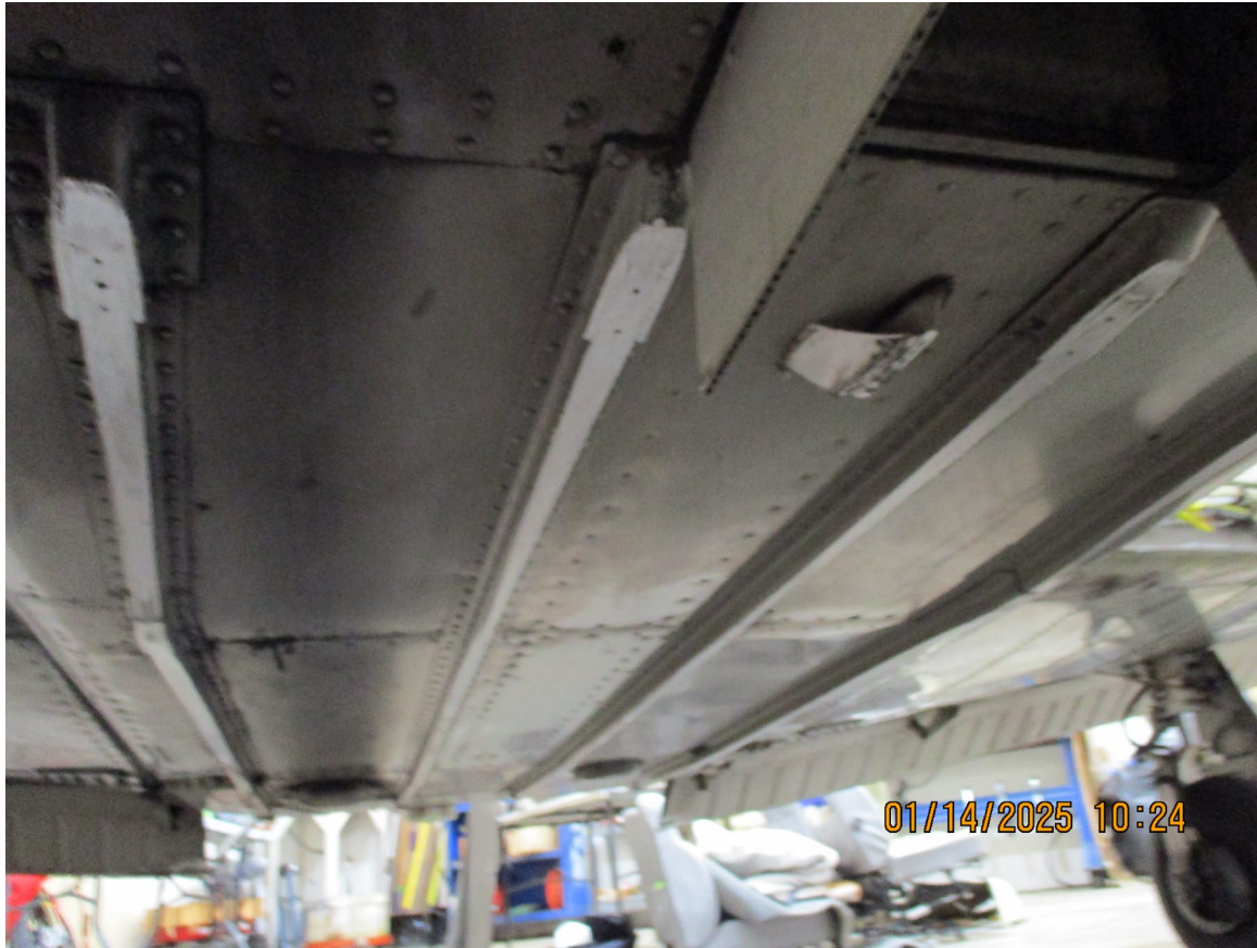
Photograph 2 - Lower fuselage accident damage (Courtesy of FAA)
