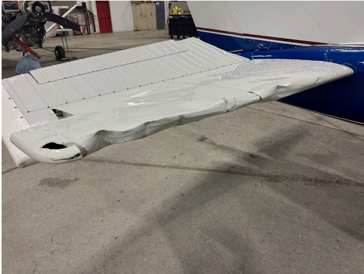
Photograph 1 - Right horizontal stabilizer accident damage (Courtesy of Pilot)
