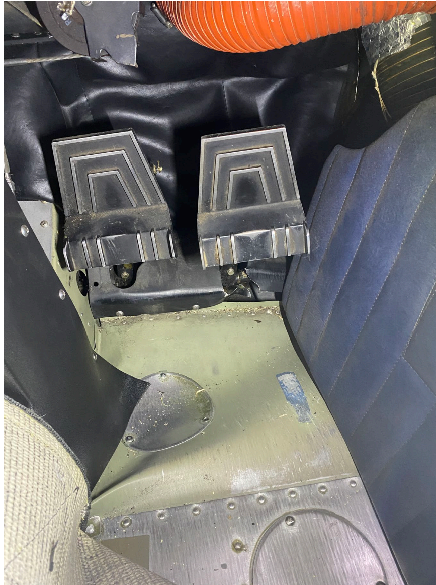
Photograph 2 - Deformation noted to copilot's floorboard structure (Courtesy of FAA)
