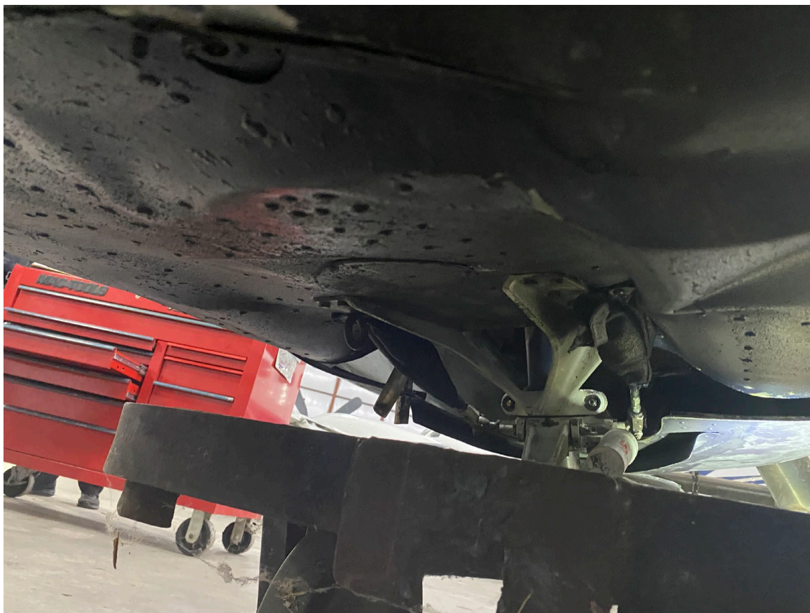
Photograph 1 - Deformation noted to lower fuselage Structure (Courtesy of FAA)
