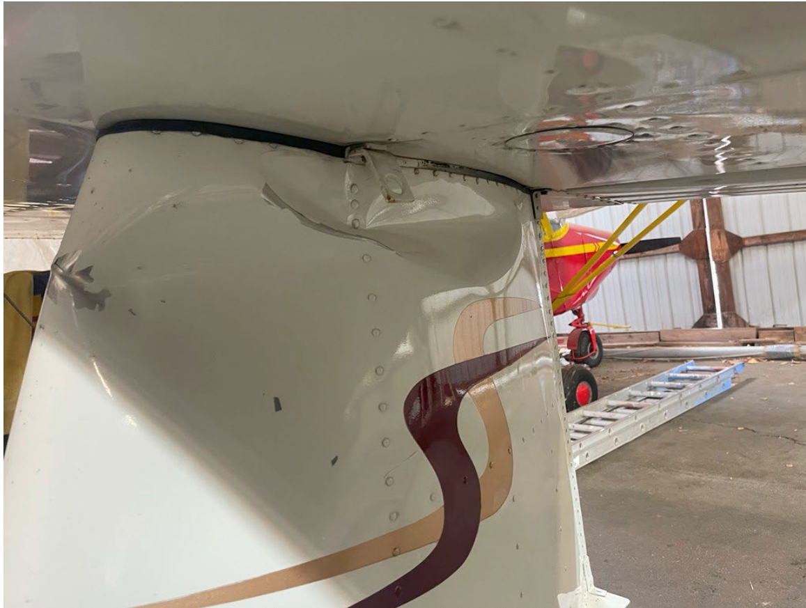
Photograph 3 - Lower Right Wing Damage (Courtesy of FAA)
