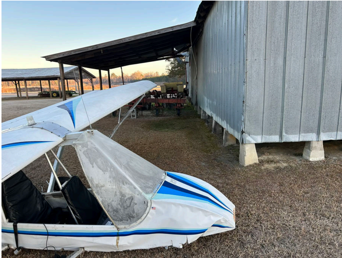
Photograph 2 - Forward right fuselage accident damage (Courtesy of FAA)
