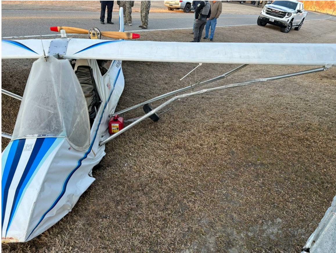
Photograph 3 - Left side wing strut accident damage, fwd and aft (Courtesy of FAA)
