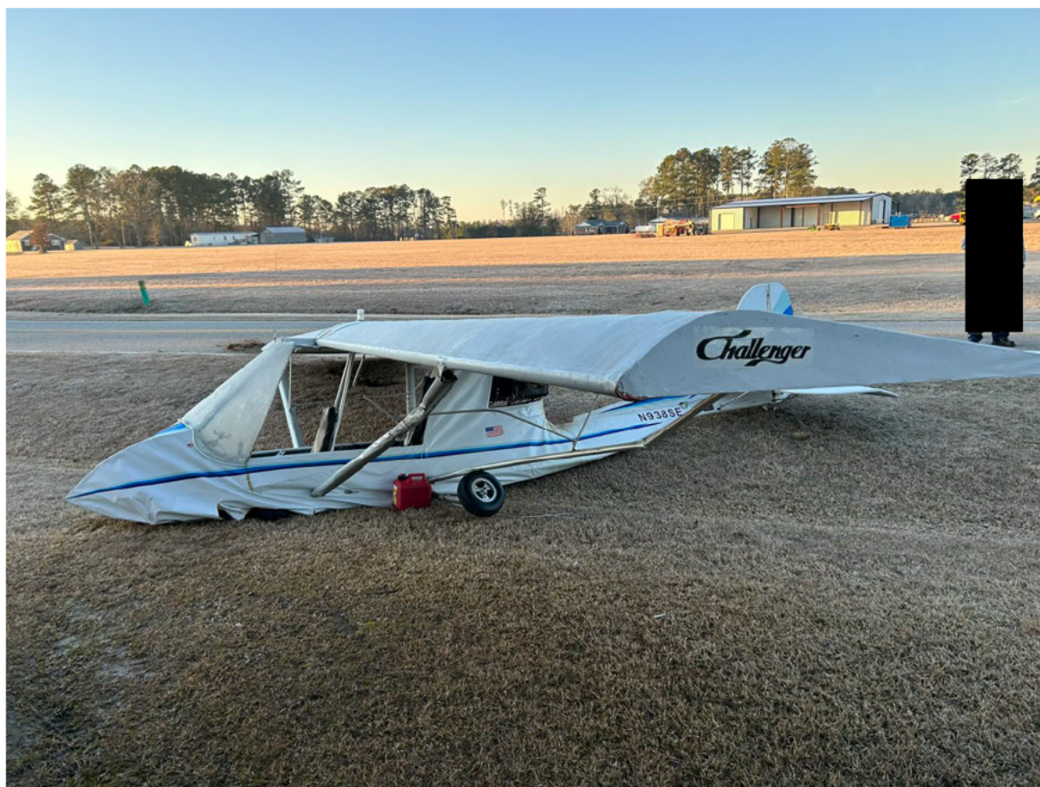
Photograph 4 - Left side fuselage accident damage (Courtesy of FAA)
