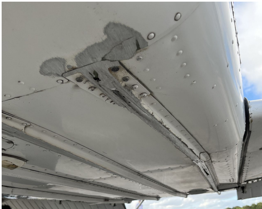
Photograph 8 - Abrasion Damage to External Longerons on the Bottom of the Fuselage. (Courtesy of FAA)
