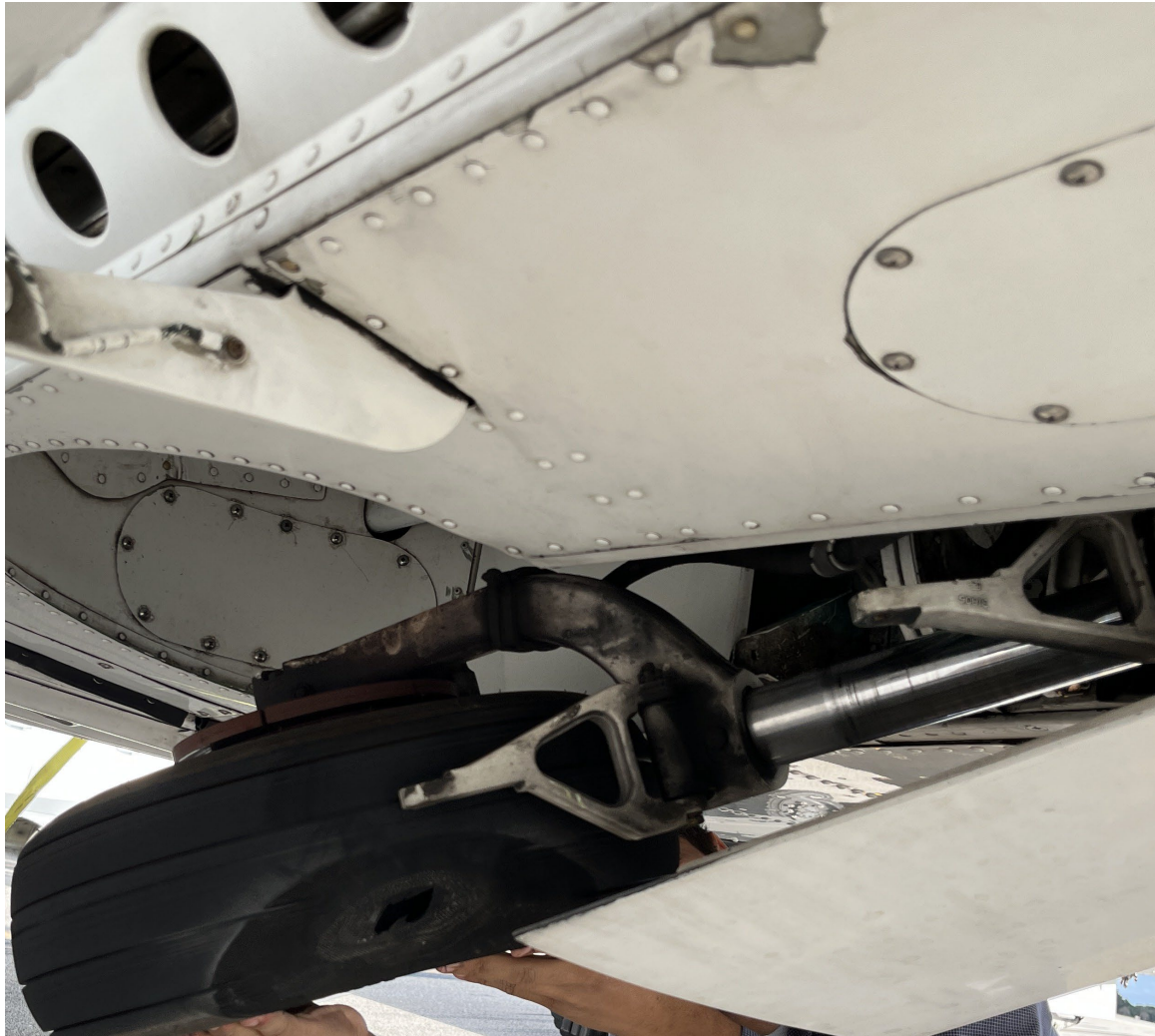
Photograph 7 - View Showing Separated Upper and Lower Torque Links of Right Main Landing Gear (Courtesy of FAA)
