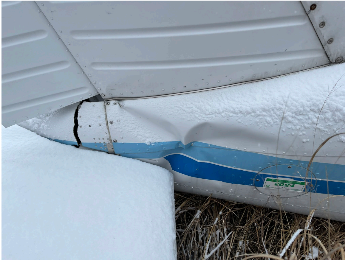
Photograph 4 - View of the empennage buckling (Courtesy of FAA)
