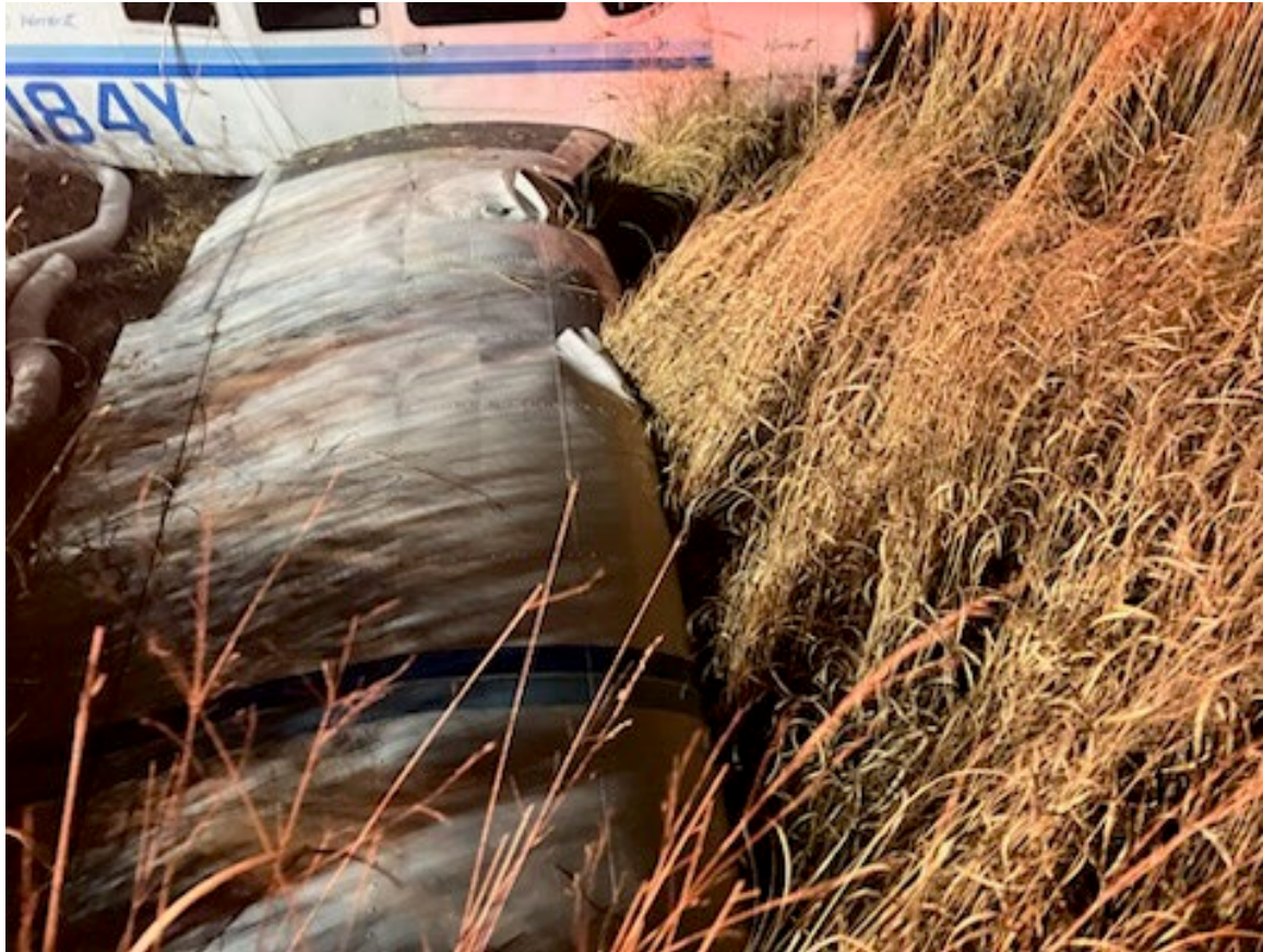
Photograph 3 - View of right wing buckling (Courtesy of FAA)
