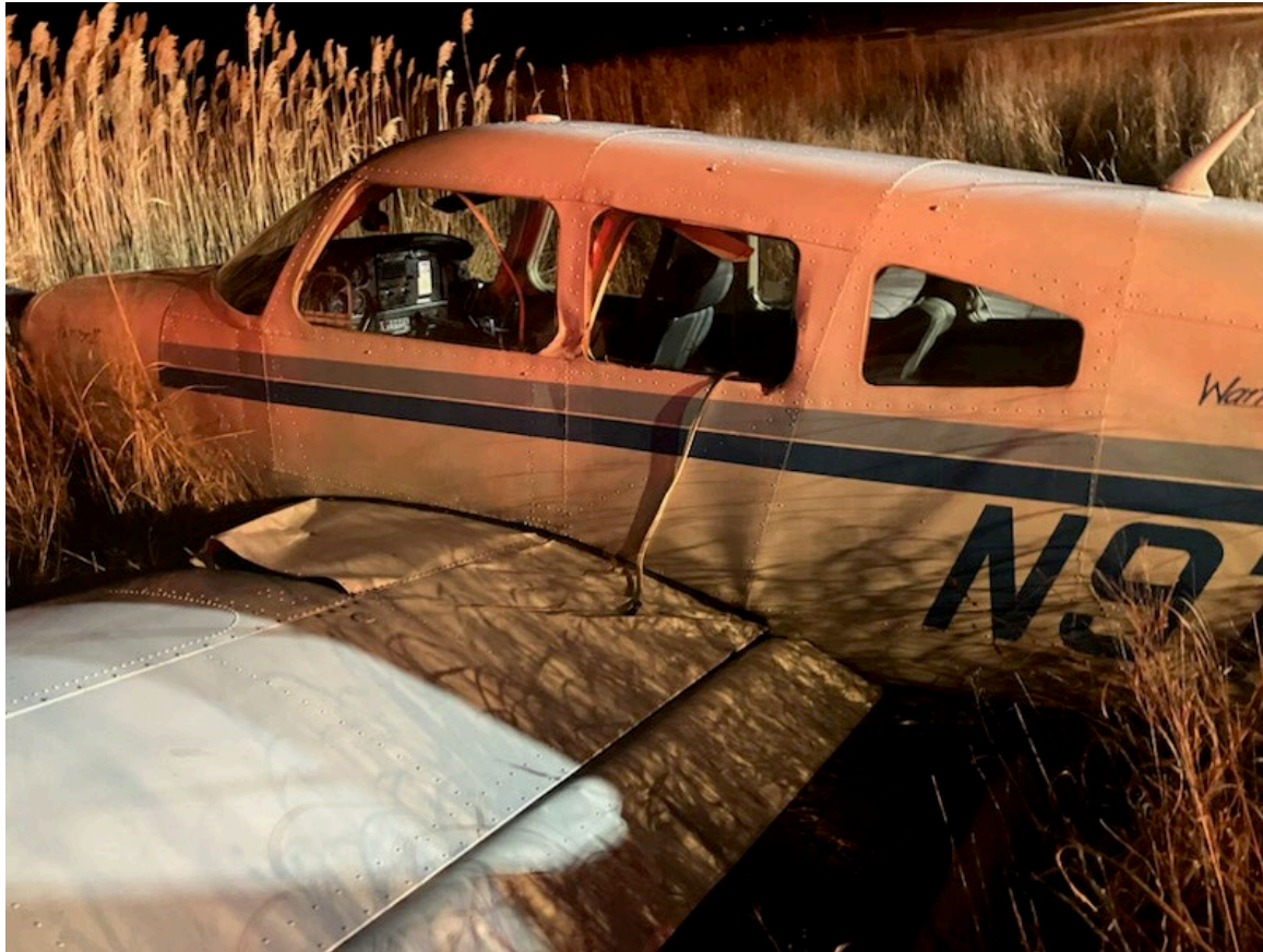
Photograph 2 - View of left-wing root buckling (Courtesy of FAA)
