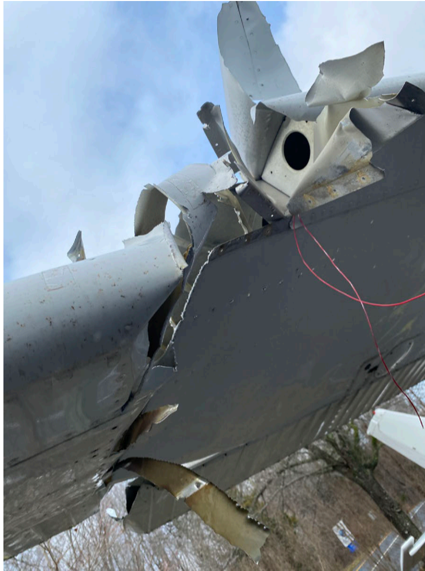
Photograph 2 - Lower right wing damage of the high wing airplane (Courtesy of FAA)
