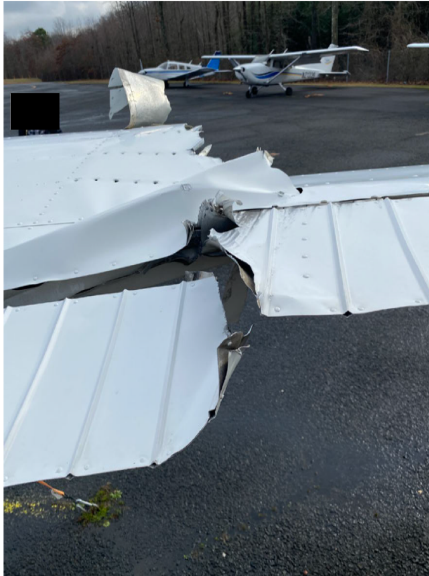
Photograph 3 - Upper right wing and aileron damage to the high wing airplane (Courtesy of FAA)
