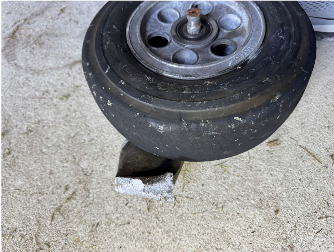
Photograph 5 - Separated nose wheel with partial fork (Courtesy of Pilot)
