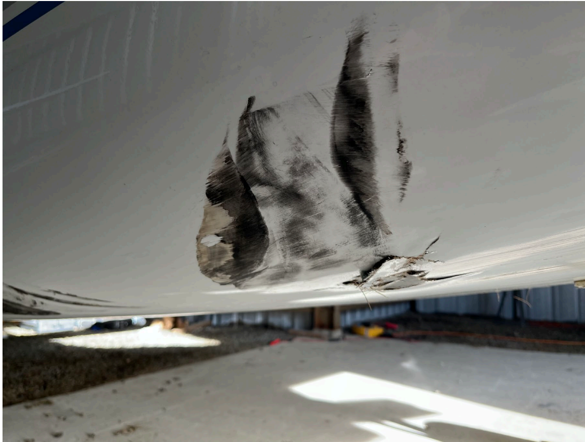
Photograph 3 - Left side fuselage damage (Courtesy of FAA)
