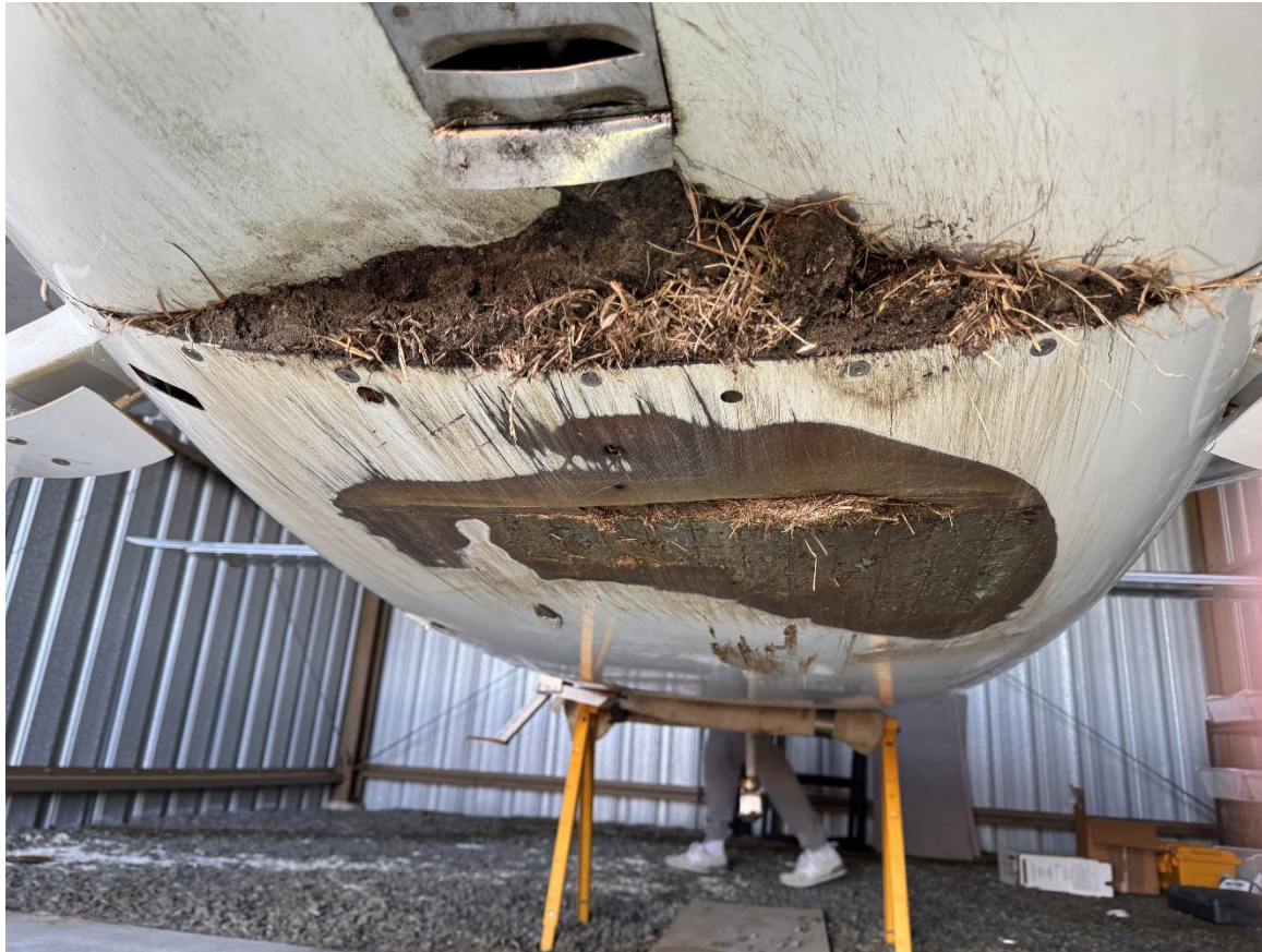
Photograph 4 - Aft belly damage (Courtesy of Pilot)
