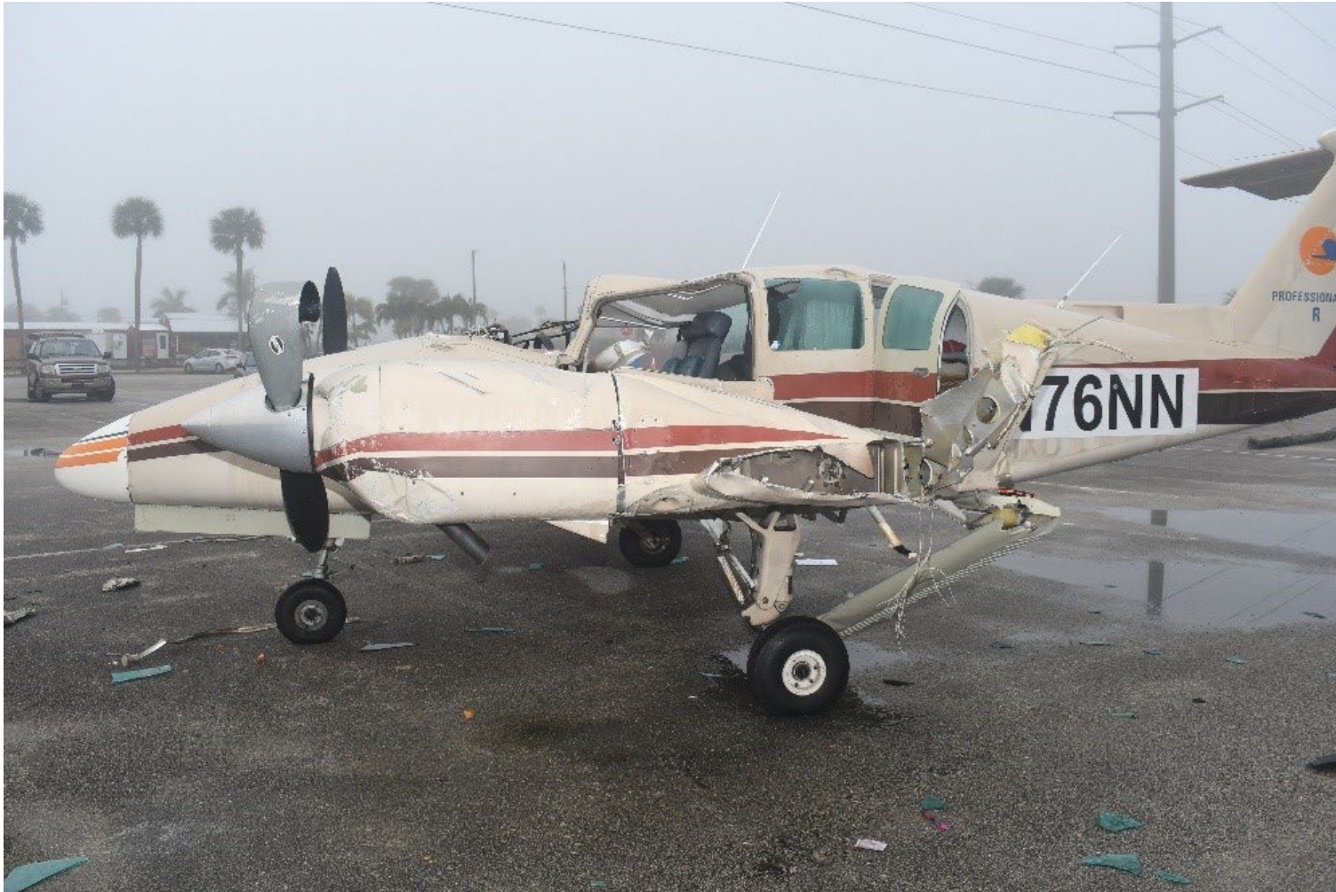
Photograph 5 - Left Wing Damage (Courtesy FAA)
