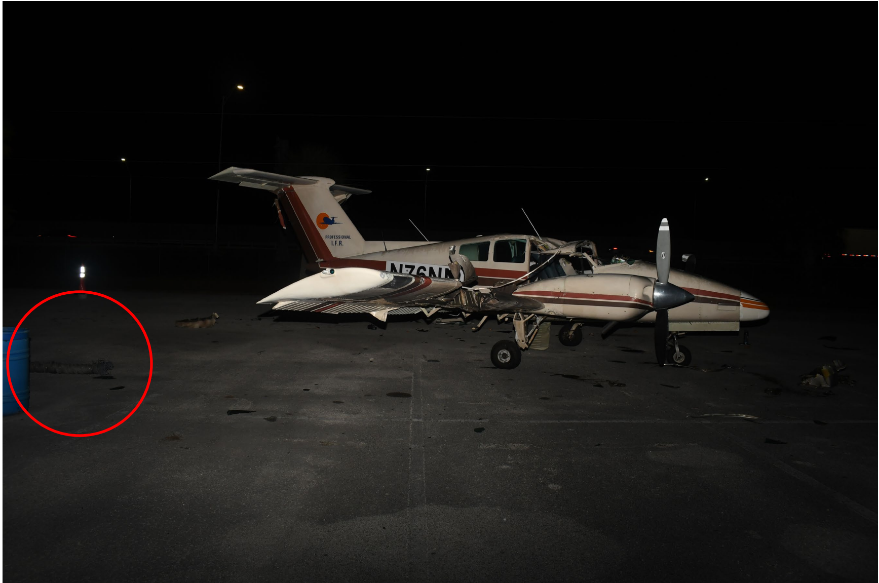
Photograph 3 - Right Side Damage and Cut Power Line (Courtesy of Melbourne PD)
