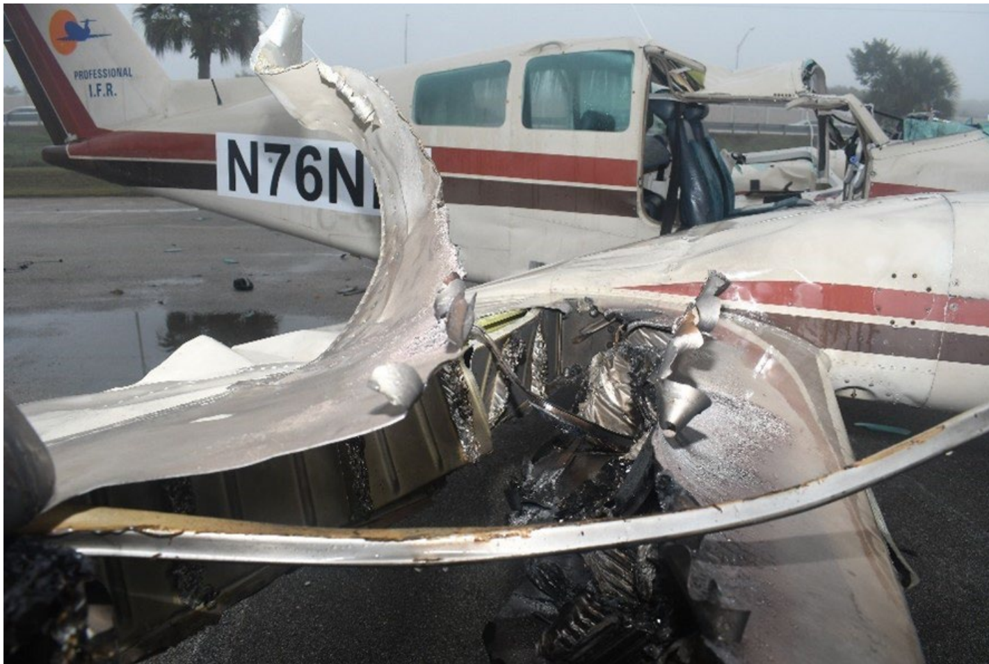
Photograph 4 - Right Wing Damage (Courtesy FAA)
