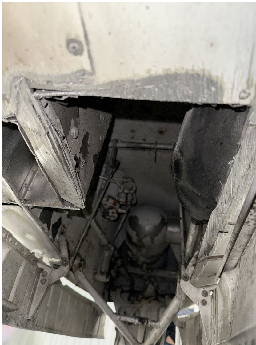
Photograph 3 - Fuselage damage (Courtesy of FAA)
