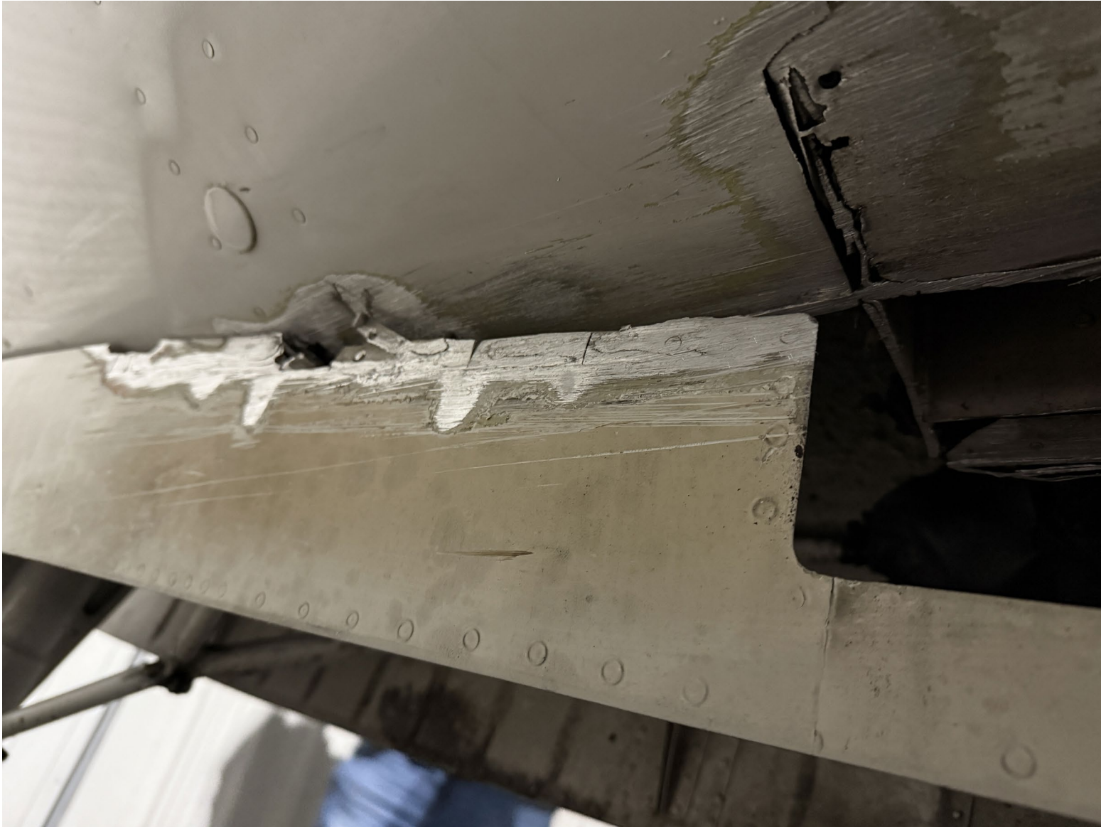
Photograph 2 - Fuselage damage (Courtesy of FAA)
