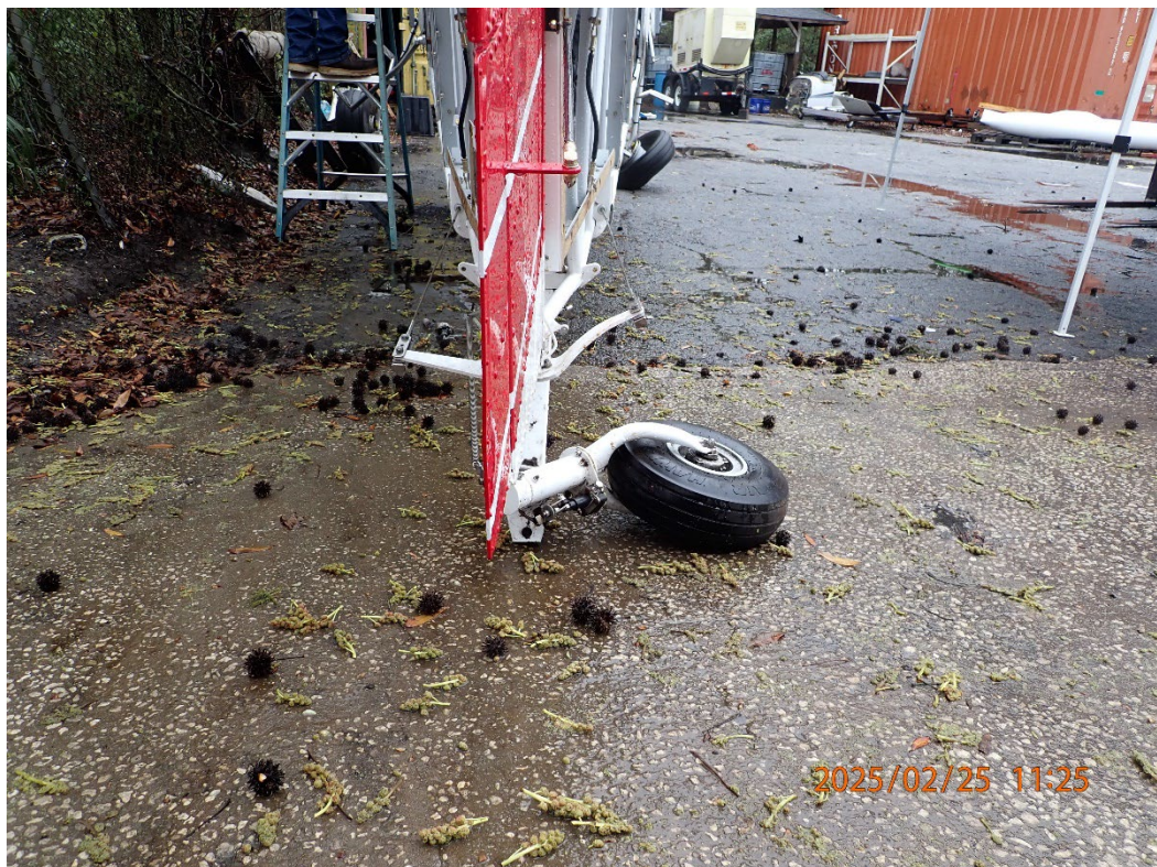
Photo 9: View of the rudder horn when bent down towards a normal position.
