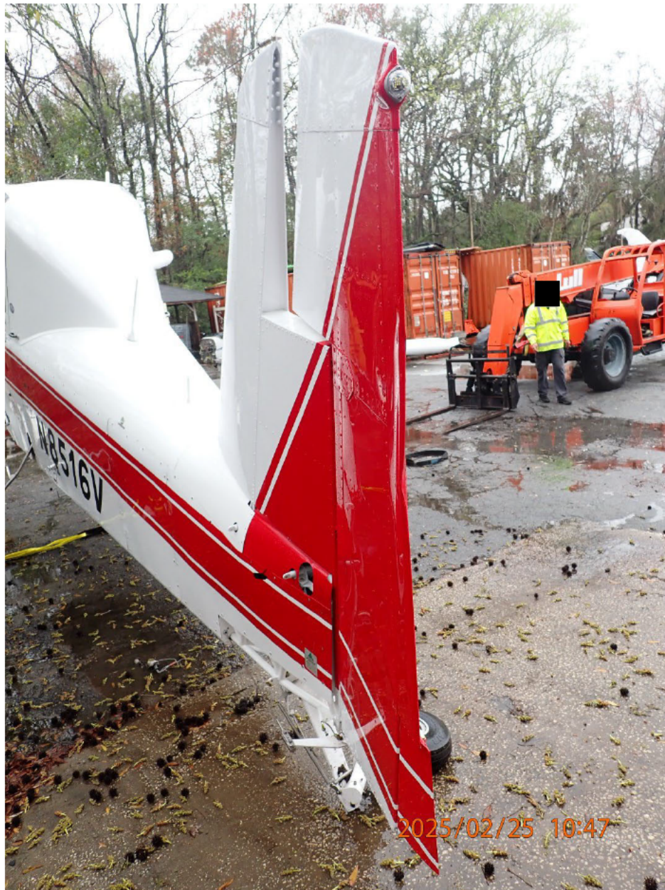
Photo 6: View of the left side of the vertical stabilizer and rudder.
