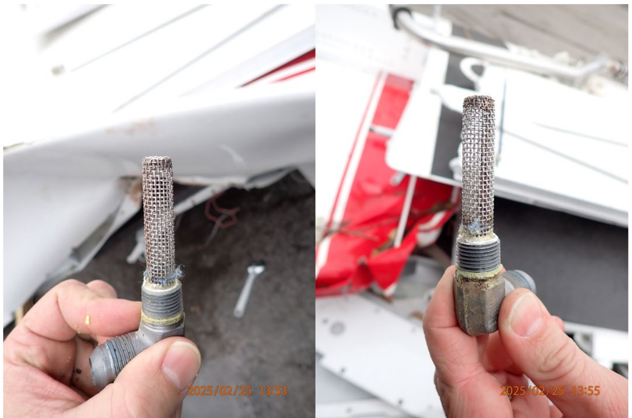
Photo 22: Fuel filter screens from the wing fuel tanks.
