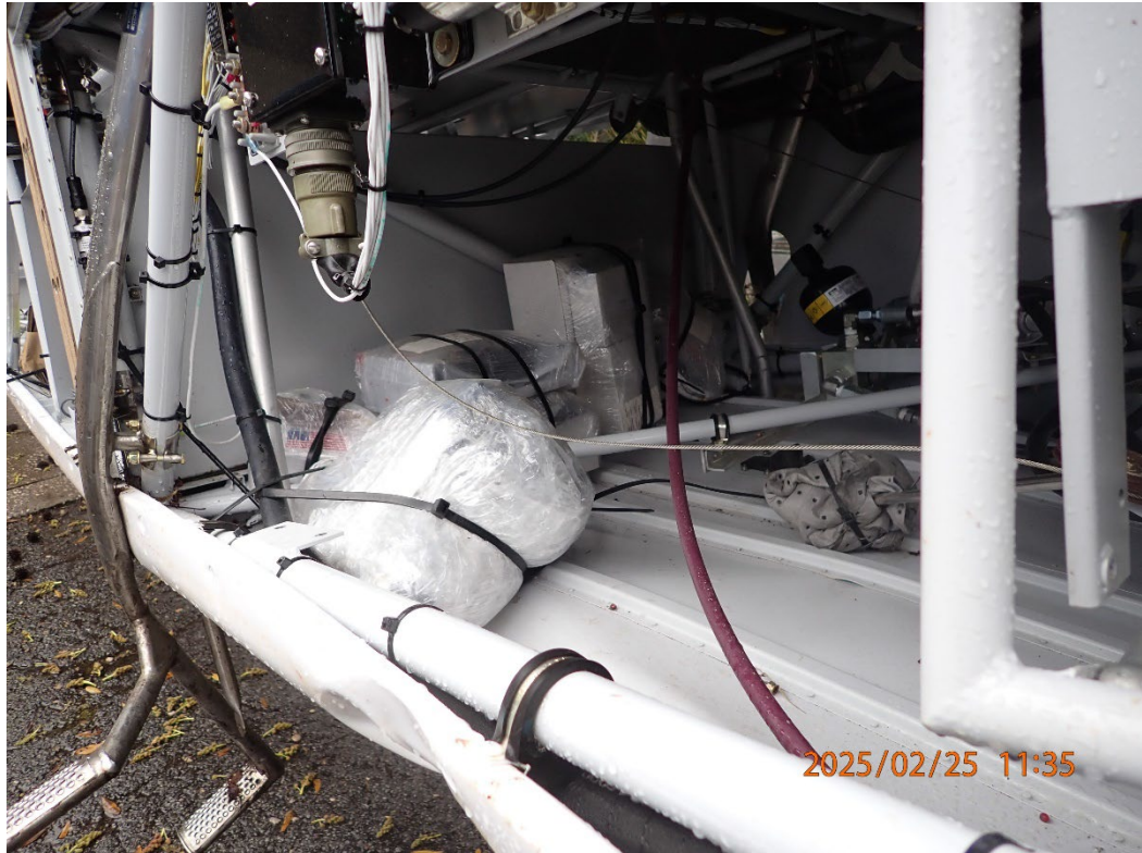
Photo 3: View of baggage under the cockpit zip tied to the tubular fuselage frame.
