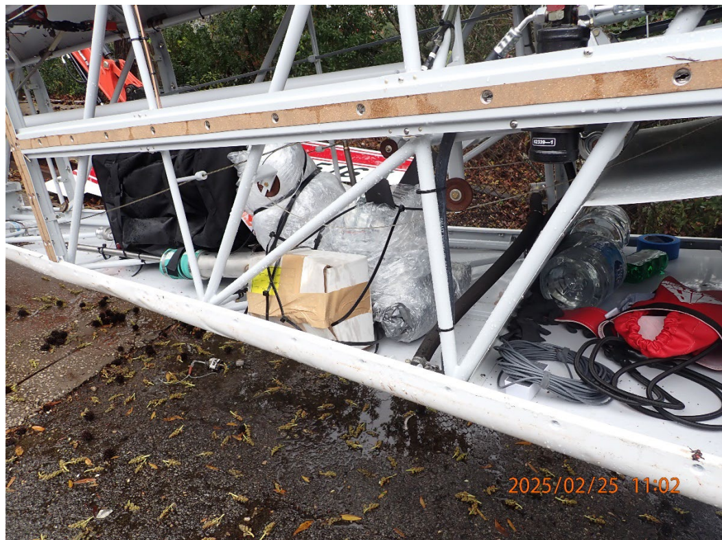
Photo 2: View of baggage zip-tied to the tubular fuselage frame.
