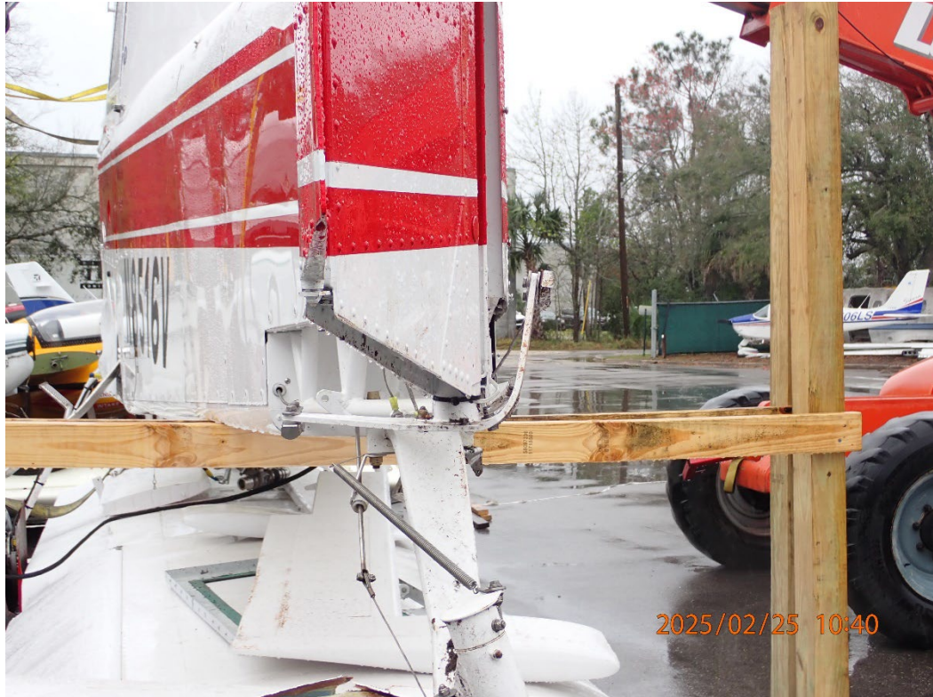
Photo 8: View of the rudder horn as first observed.
