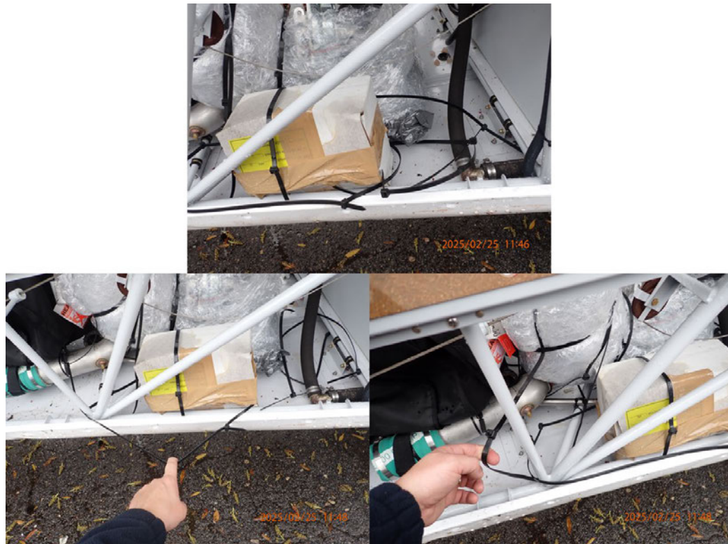
Photo 5: View of cut and loose zip ties in the aft fuselage area.
