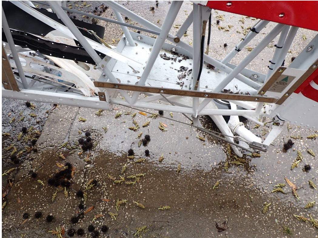
Photo 13: View of the left side rudder cables.
