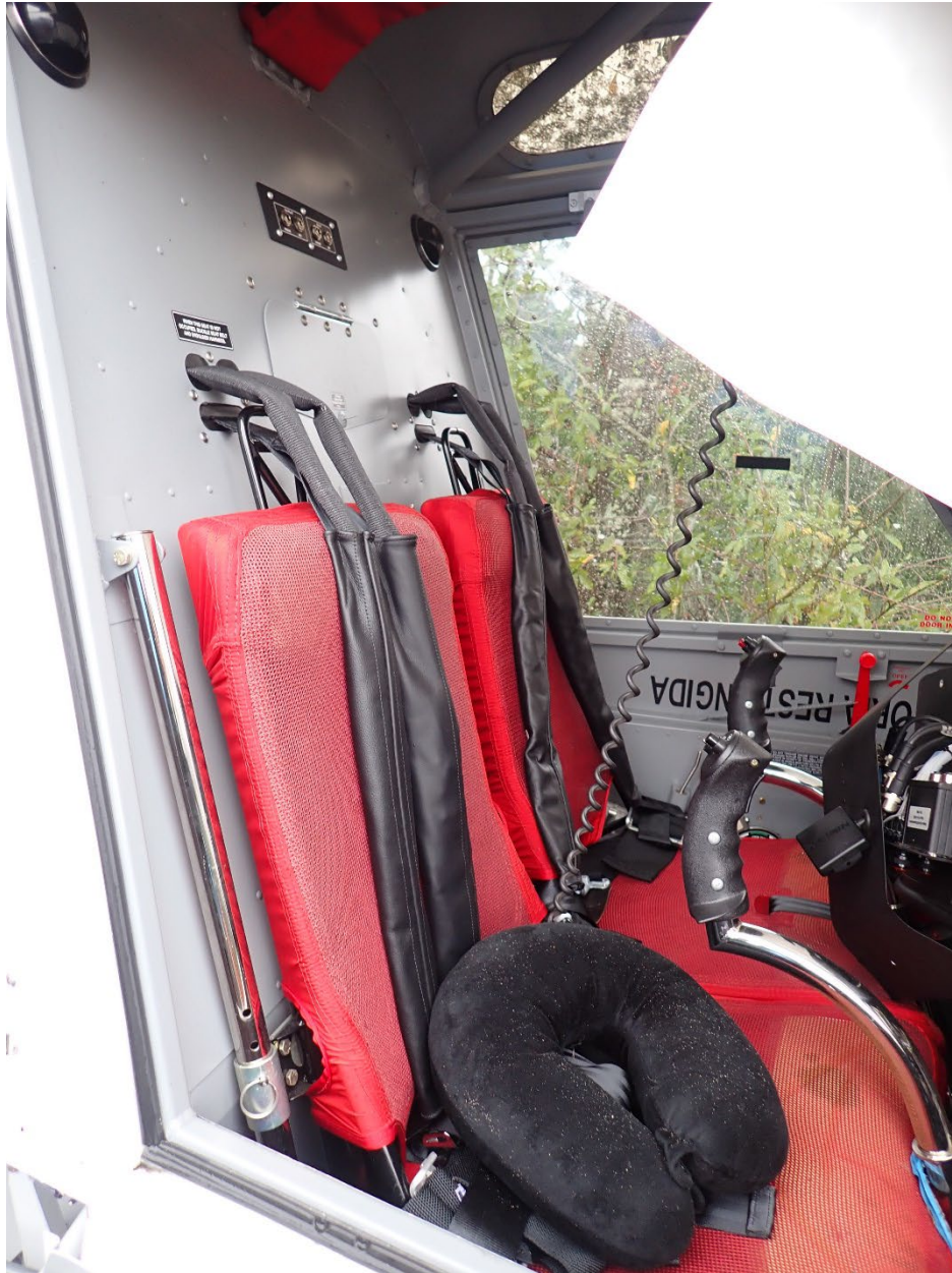
Photo 20: View of the cockpit with harness airbags not deployed.
