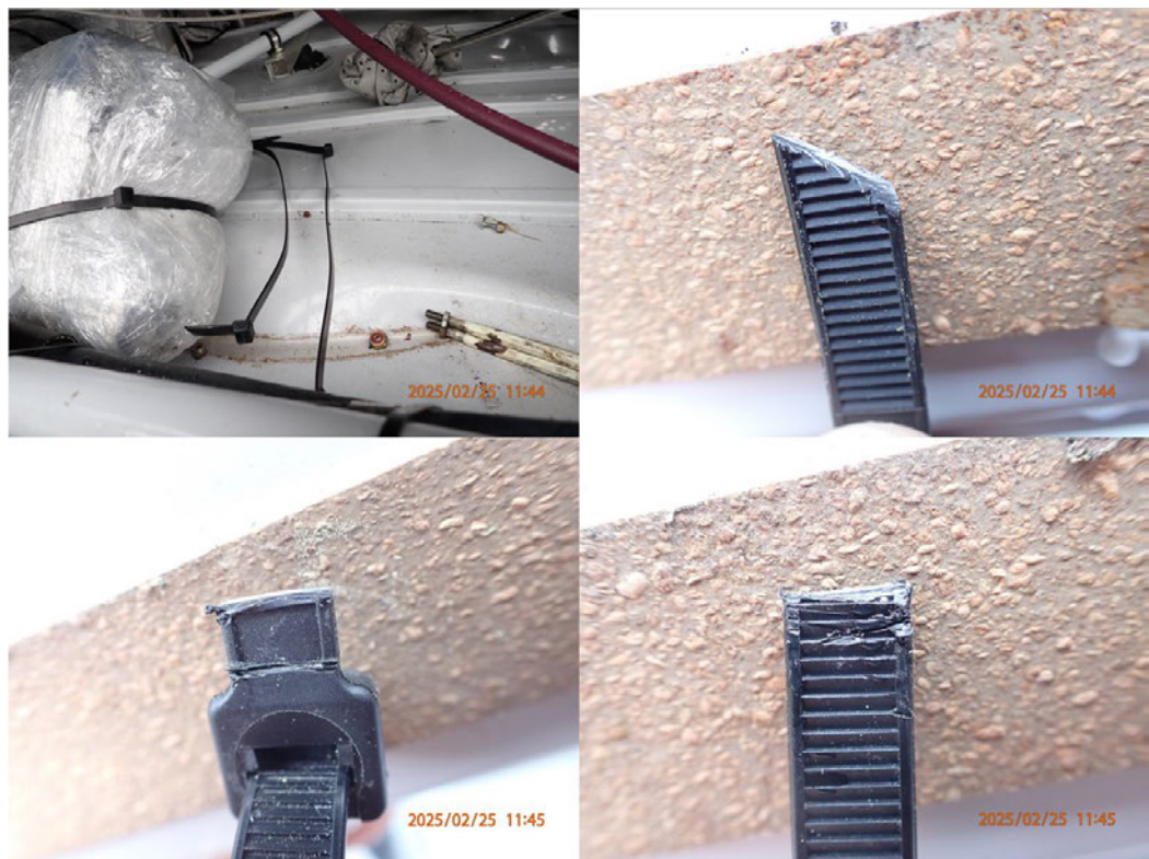
Photo 4: View of cut zip ties from under the cockpit area.
