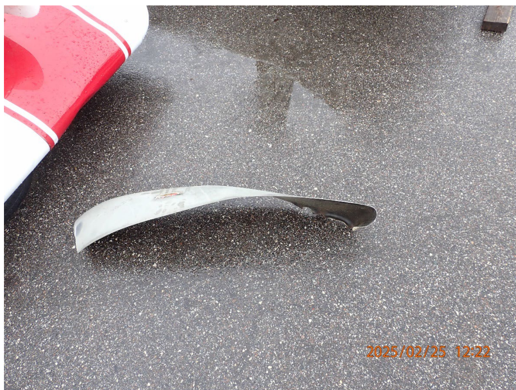
Photo 25: View of the propeller blade cut by recovery crews.
