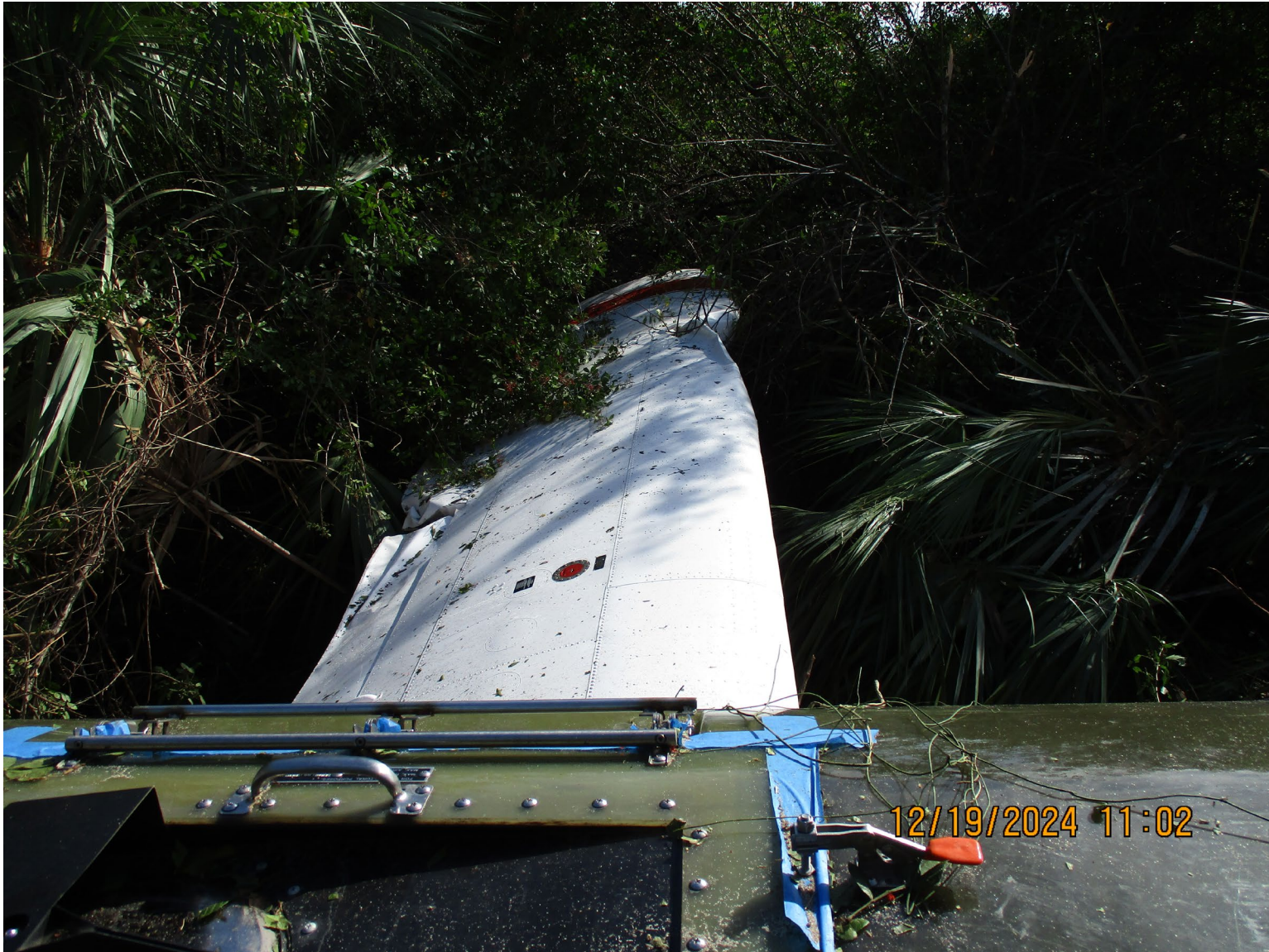
Photograph 4 - View of damage to the left wing. (Courtesy of FAA)
